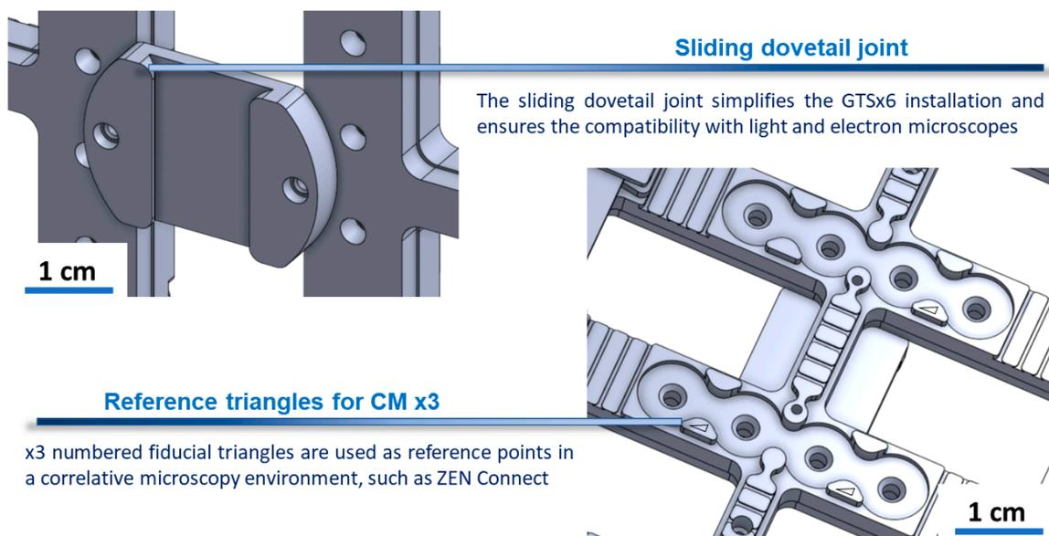
**Figure 2. Innovative sample holder design compatibility and calibration.** The holder features three numbered fiducial markers (reference triangles) for ZEN Connect software alignment and a sliding dovetail joint for easy installation and microscope compatibility.
