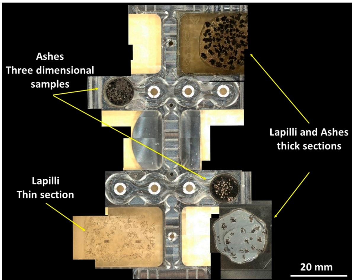
**Figure 3.** Acquisition of reference images for the application of the CLEM workflow. Multiple reference images of the GTSx6 sample holder with the specimens mounted on it were acquired using LM. Lapilli and ashes thick/thin sections, as well as three-dimensional samples, were investigated.
