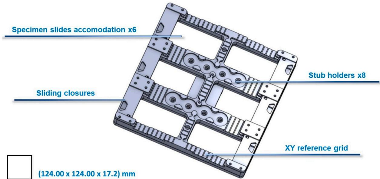
**Figure 1. Innovative sample holder design features.** GTSx6 sample holder accommodates six specimen slides and features six sliding closures for optimal sample stabilization. The holder is provided with eight stub holders for positioning additional samples and/or standards used in chemical analysis. GTSx6 also includes an XY reference grid and three fiducial markers for easy calibration and alignment using ZEN Connect software.
