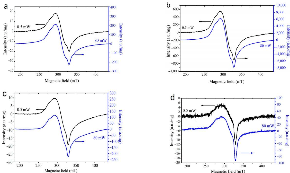
**Figure 11.** EPR spectra of the samples synthesized using  $\text{CuHPO}_4 \cdot \text{H}_2\text{O}$  (a),  $\text{CuO}$  (b),  $\text{Cu}_2\text{O}$  (c) and  $\text{Cu}$  (d) at  $x = 1$ , at different powers of microwave irradiation.
