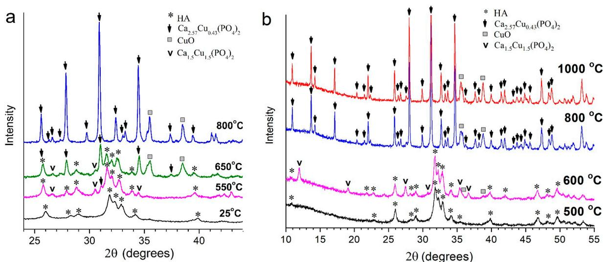
**Figure 15.** In situ (a) and ex situ (b) XRD patterns of Cu-HA sample, synthesized with copper phosphate content  $x = 2$ .
