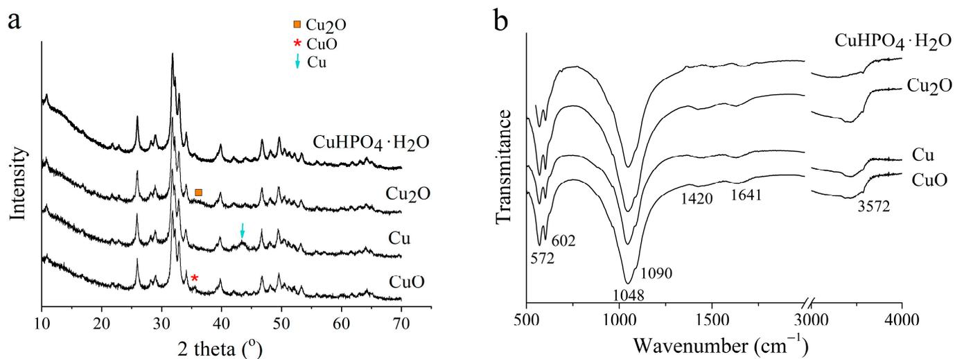
**Figure 6.** XRD patterns (a) and FTIR spectra (b) of Cu-HA samples with different sources of Cu at x = 1 and mechanochemical treatment for 25 min.
