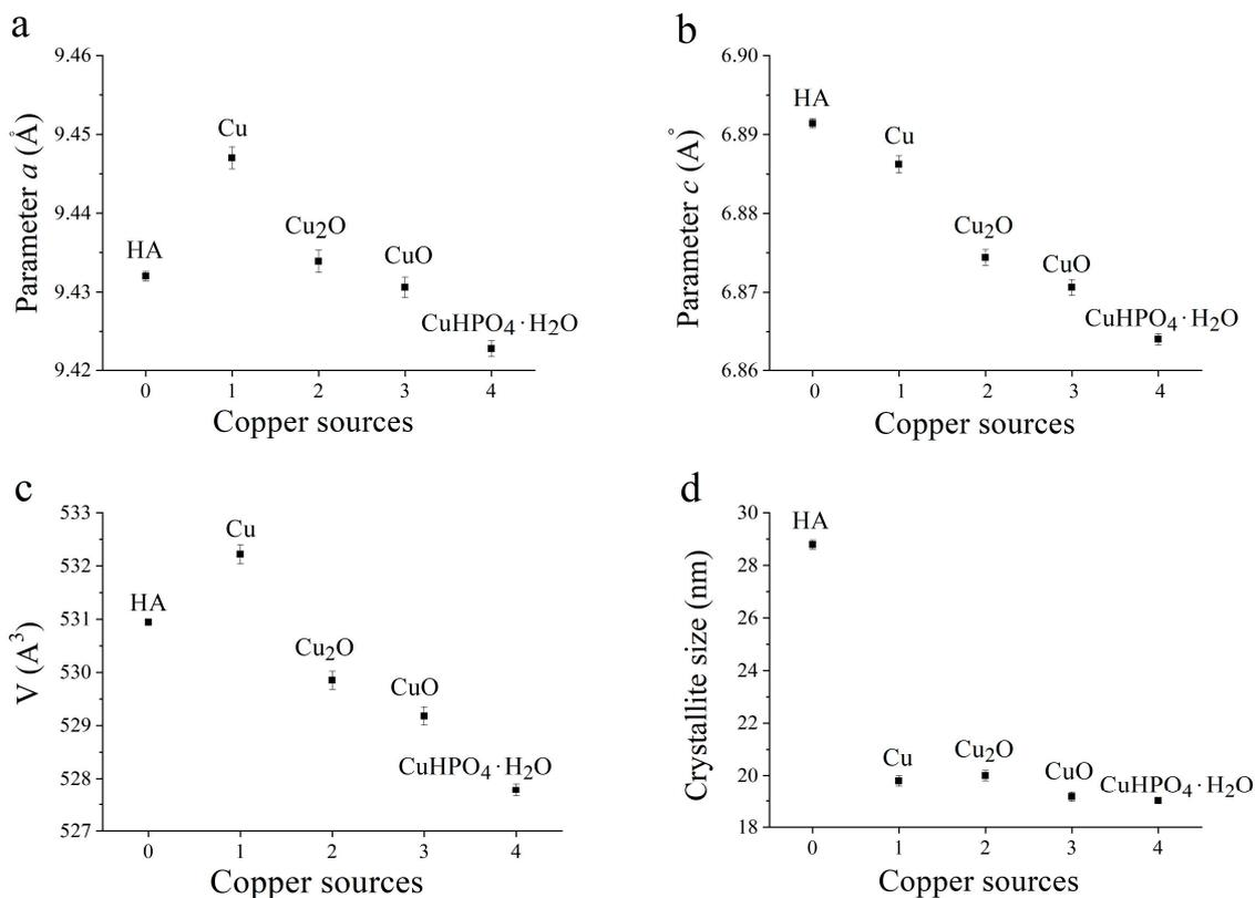
**Figure 8.** A comparison of unit cell parameters  $a$  (a) and  $c$  (b), cell volume (c), and crystallite size (d) in Cu-HA for syntheses from different copper sources at concentration  $x = 1$ . Duration of mechanochemical treatment for all the samples is 25 min.
