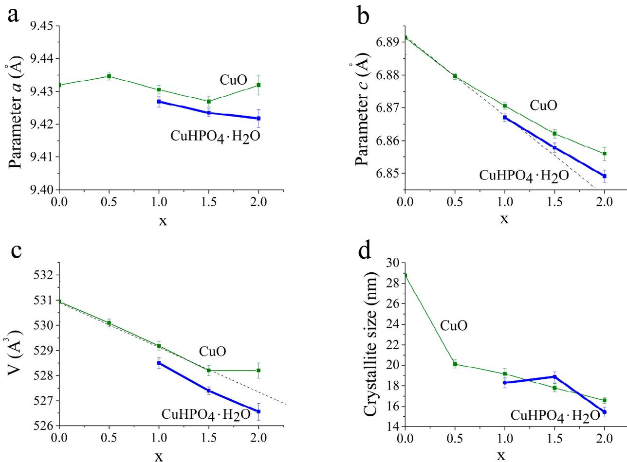
**Figure 5.** Changes in parameters *a* (a) and *c* (b) of the HA unit cell, volume (c), and crystallite size (d) with an increase in the concentration of the initial CuO or CuHPO<sub>4</sub>·H<sub>2</sub>O.
