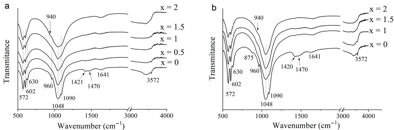
**Figure 4.** FTIR spectra of samples containing different concentrations of initial CuO (a) or  $\text{CuHPO}_4 \cdot \text{H}_2\text{O}$  (b), after mechanochemical treatment for 25 min.
