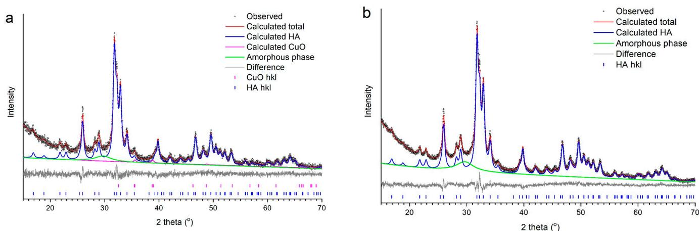
**Figure 3.** Full-profile Rietveld decomposition of XRD patterns of as-synthesized Cu-HA samples using CuO (a) and  $\text{CuHPO}_4 \cdot \text{H}_2\text{O}$  (b) with the same copper concentration ( $x = 1$ ). Duration of mechanochemical treatment for both samples was 25 min.
