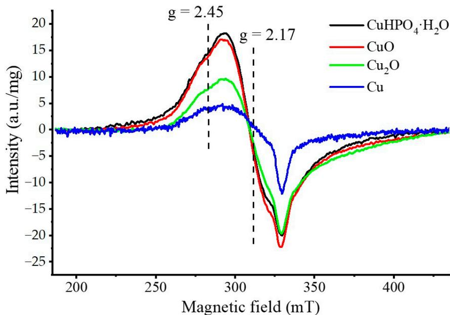
**Figure 10.** EPR spectra of the samples synthesized using different copper sources at concentration  $x = 1$ . Microwave power is 0.5 mW.
