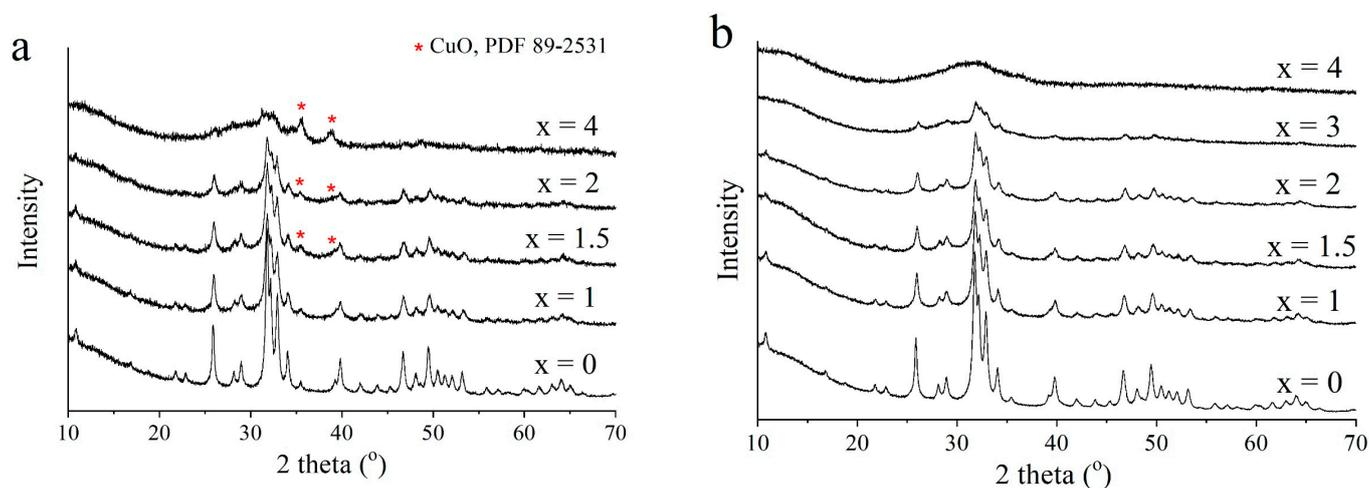
**Figure 2.** XRD patterns of samples containing different concentrations of initial CuO (a) or  $\text{CuHPO}_4 \cdot \text{H}_2\text{O}$  (b) after mechanochemical treatment for 25 min.
