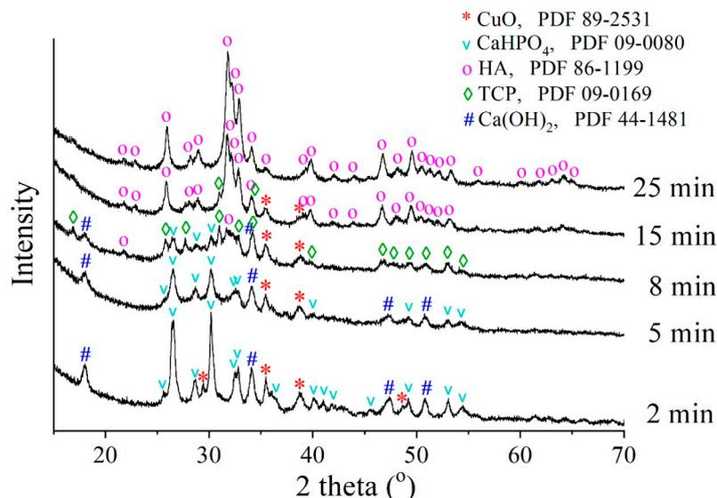
**Figure 1.** XRD patterns of the reaction mixture containing CuO at  $x = 1$  after mechanochemical treatment for different periods.
