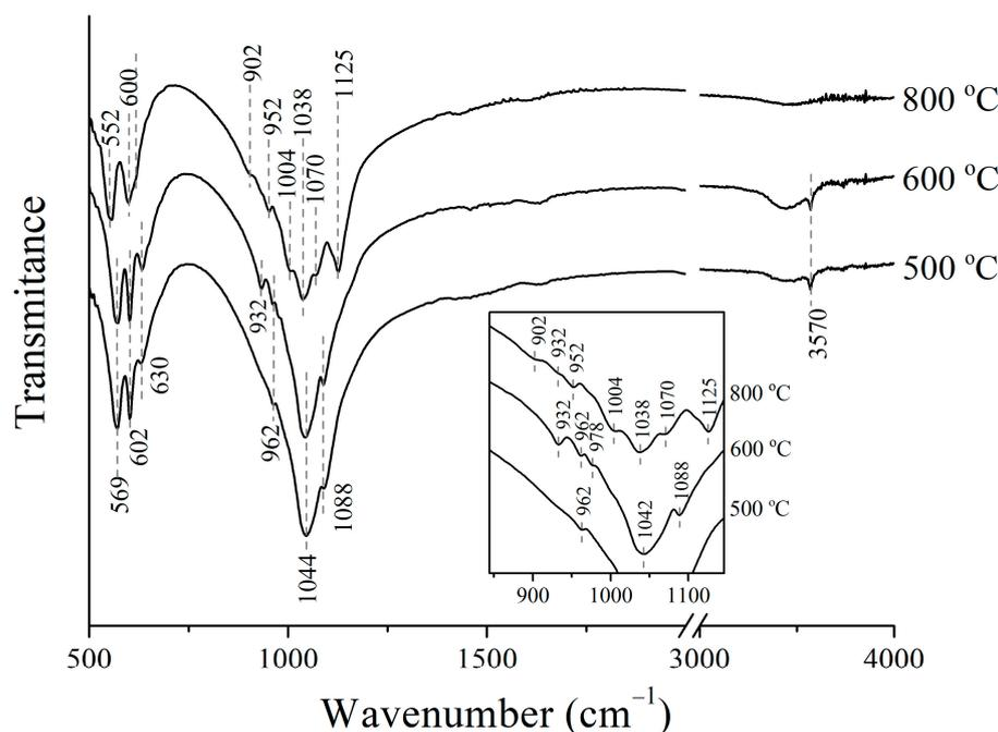
**Figure 16.** FTIR spectra of the heated Cu-HA samples with copper phosphate content  $x = 2$ .
