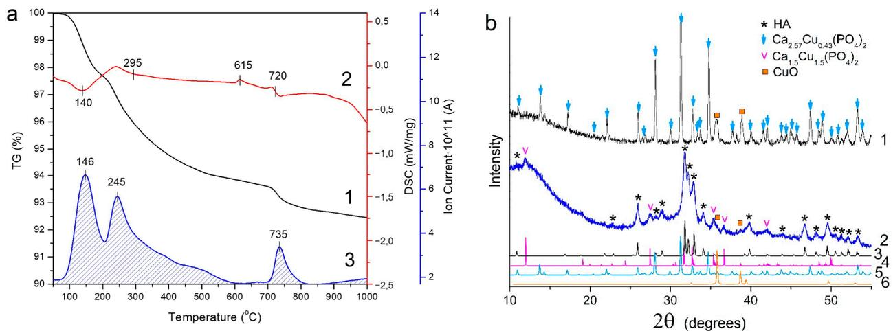
**Figure 14.** STA (a) of Cu-HA sample with copper phosphate content  $x = 2$ ; 1—mass loss; 2—DSC; 3—evolution of water. XRD patterns (b) of the sample after STA upon heating up to 1000 °C (1) and 640 °C (2) in comparison with modeled patterns from the PDF database: 3—HA, PDF 000-86-1199; 4— $\text{Ca}_3\text{Cu}_3(\text{PO}_4)_4$ , PDF 000-72-0203; 5— $\text{Ca}_{18}\text{Cu}_3(\text{PO}_4)_{14}$ , PDF 000-53-0171; 6—CuO, PDF 000-89-2531.
