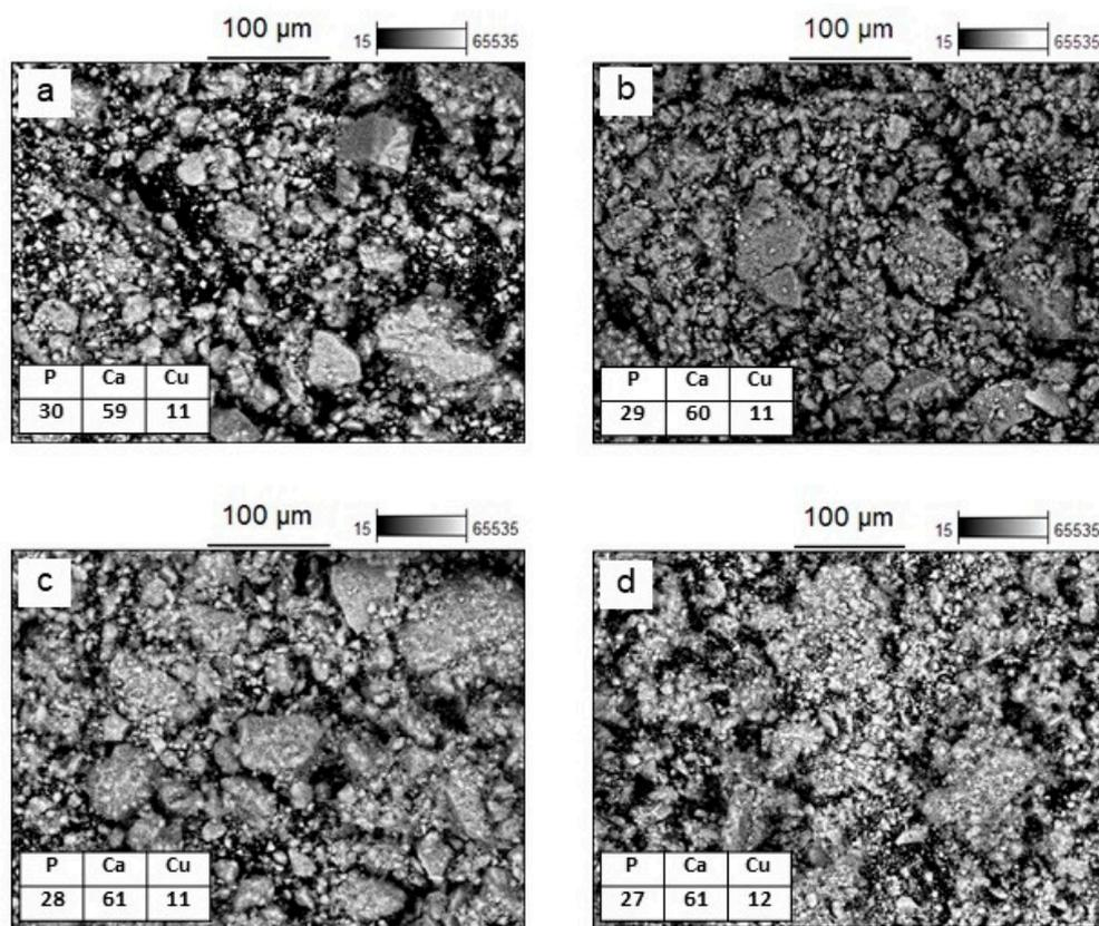
**Figure 9.** SEM images of powder morphology of the Cu-HA samples synthesized using CuO (a),  $\text{CuHPO}_4 \cdot \text{H}_2\text{O}$  (b),  $\text{Cu}_2\text{O}$  (c) and Cu (d) at concentration  $x = 1$ . Duration of mechanochemical treatment for all samples is 25 min. The tables show the weight concentrations of the registered elements at the semiquantitative EDX analysis of these areas.
