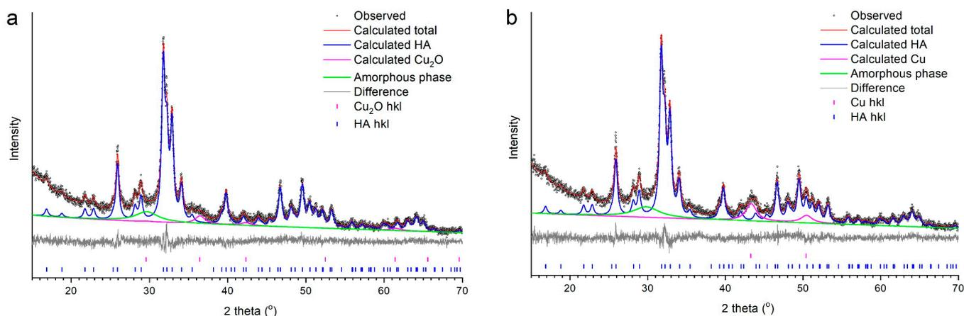
**Figure 7.** Full-profile Rietveld refinement of XRD patterns of Cu-HA samples synthesized using  $\text{Cu}_2\text{O}$  (a) and Cu (b) at concentration  $x = 1$ . Duration of mechanochemical treatment for both samples is 25 min.
