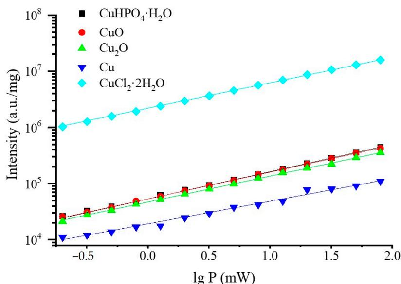
**Figure 12.** Integral intensities of the EPR signal of  $\text{CuCl}_2 \cdot 2\text{H}_2\text{O}$  and the samples synthesized using different copper sources ( $x = 1$ ) as a function of the power of microwave irradiation.
