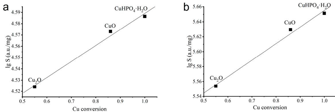
**Figure 13.** Decimal logarithm of the integral intensity of the EPR signal ( $\lg S$ ) at 0.5 mW (a) and 80 mW (b) on the degree of copper conversion according to XRD data (Table 1).
