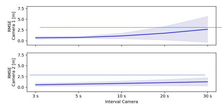
**Figure 14.** Mean RMSD (solid blue line) and standard deviation (shaded areas), for intervals of 3 s, 5 s, 10 s, 20 s, and 30 s, compared to 1 s interval, for (**Top**) Camera 1 and (**Bottom**) Camera 2.
