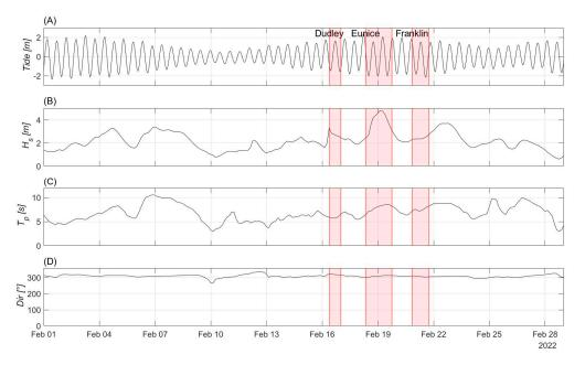
**Figure 2.** Hydrodynamics during the monitoring period with in (**A**) tidal elevation, (**B**) significant wave height, (**C**) peak wave period, and (**D**) mean wave direction, from shallow-water SWAN datapoint. Source: Marine Institute.
