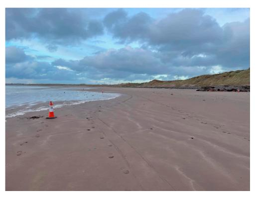
Figure 5. Road traffic cones were placed in the field and used as temporary GCPs.
