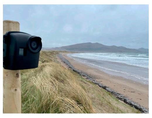
Figure 4. Photo of Brinno TLC2000 Camera 1 deployed in the field.
