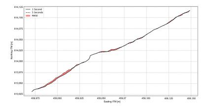
**Figure 11.** Example of RMSD between shoreline edge detected on Timex with 1 s interval (solid line) and 5 s interval (dashed line) from 26 February 2022 at high tide. The red area represents the RMSD between both lines.
