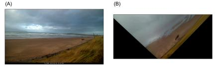
**Figure 13.** Example of (**A**) snapshot and (**B**) resulting Timex image during receding tides, showing remaining water on the beach face resulting in shoreline edge detection not representing the actual shoreline (from 26 February 2022 at 10 h).
