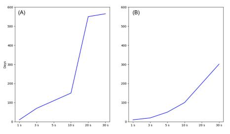
**Figure 15.** (**A**) Average battery life for the different intervals, and (**B**) average days that SD card can be used for the different intervals, from Brinno (2022).
