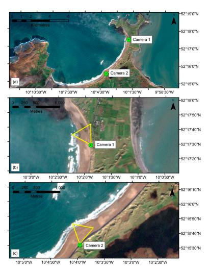
**Figure 3.** (a) Overview of Brandon Bay with the location of both cameras; (b) detail of the field of view of Camera 1, represented by the yellow triangle; and (c) detail of the field of view of Camera 2, on a satellite image (from ESA—Sentinel 2).
