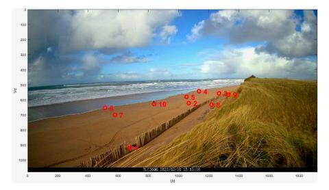
Figure 6. Temporary GCPs used in the field (Camera 2), with the red circles representing the GCPs.
