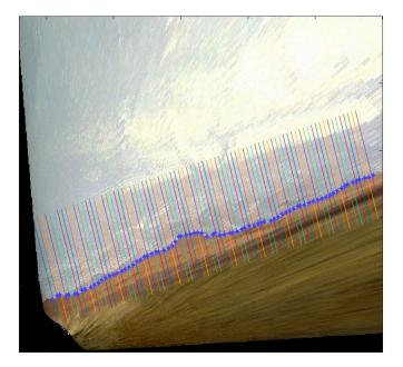
**Figure 8.** Transects covering the swash zone in front of Camera 2 (From 26 February 2022)—interval 1 s. The blue line is the detected shoreline.
