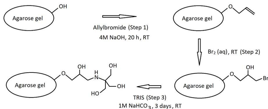
**Figure 1.** Scheme of agarose gel chemical modification with TRIS (tris-(hydroxymethyl) aminomethane).
