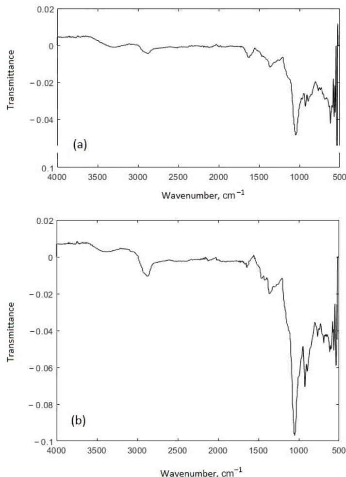
**Figure 2.** FTIR spectra of freeze-dried Zetarose FlashFlow 4 (a) and allyl-Zetarose Flash. Flow 4 (b) gels.
