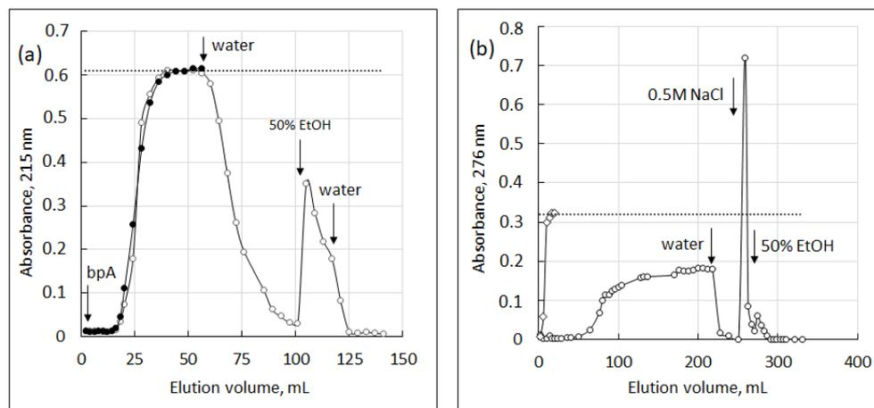
**Figure 6.** Breakthrough curves of (a) bisphenol A (10 mg/L) and (b) diclofenac (10 mg/L) obtained on 1 mL columns with TRIS-Zetarose 4FF (○). Closed circles relate to repeated application of bisphenol A to the column. (b): Breakthrough curve of diclofenac on 1 mL column with Zetarose-4FF (◇). Flow rate 0.4 mL/min. Dotted lines indicate absorbances of the starting bisphenol A and diclofenac solutions.
