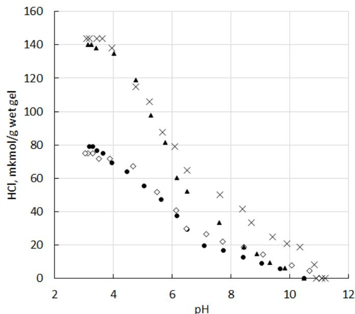
**Figure 3.** Potentiometric titration curves: (●) TRIS-Sepharose 4B, (◇) TRIS-Zetarose FlashFlow4, (▲) TRIS-ZetaCell CL6B, and (×) EA-Zetarose FlashFlow4.
