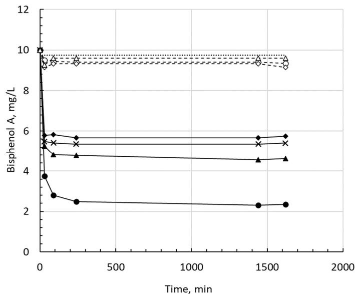
**Figure 4.** Kinetics of bisphenol A adsorption on TRIS-containing agarose gels (filled symbols) and the corresponding parent gels (open symbols). (▲)—TRIS-ZetaCell CL6B; (●)—TRIS-Sepharose 4B; (◆)—TRIS-Zetarose FF4; and (×) EA-Zetarose FF4. The gels (0.25 mL sediment) were added to 9.75 mL bisphenol A (10 mg/L). The upper dotted line designates 9.75 mg/L bisphenol A concentration resulting from diluting with 0.25 mL of water.
