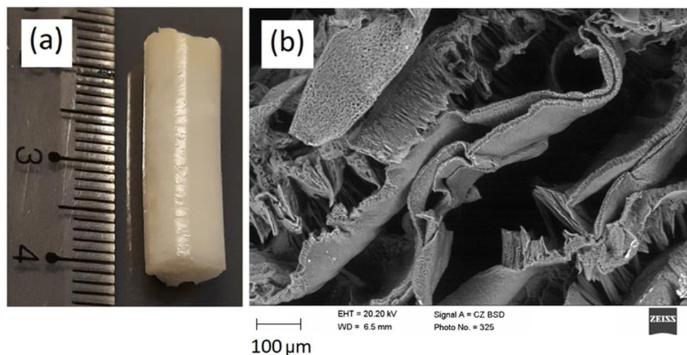
**Figure 8.** The macroscopic (a) and microscopic (b) views of poly (vinyl alcohol) cryogels produced according to the study [15]. The monolithic gel was cut perpendicular to the axis to get the slice shown in (b).
