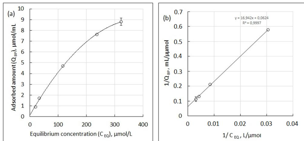
**Figure 5.** Adsorption isotherm of bisphenol A on TRIS-ZetaCell CL6B: (a)  $Q_{BP}$  as a function of  $c_{EQ}$ ; (b)  $1/Q_{BP}$  as a function of  $1/c_{EQ}$ ; and the intercept equals to  $1/Q_{max}$ . The error bars are standard deviations for two independent measurements.
