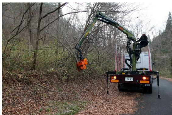
**Figure 1.** Harvesting experiment with a truck-mounted multi-tree felling head.
