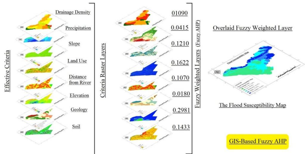
Figure 4. Classification of overlaying weighted fuzzy layers' process based on the criteria specified.
