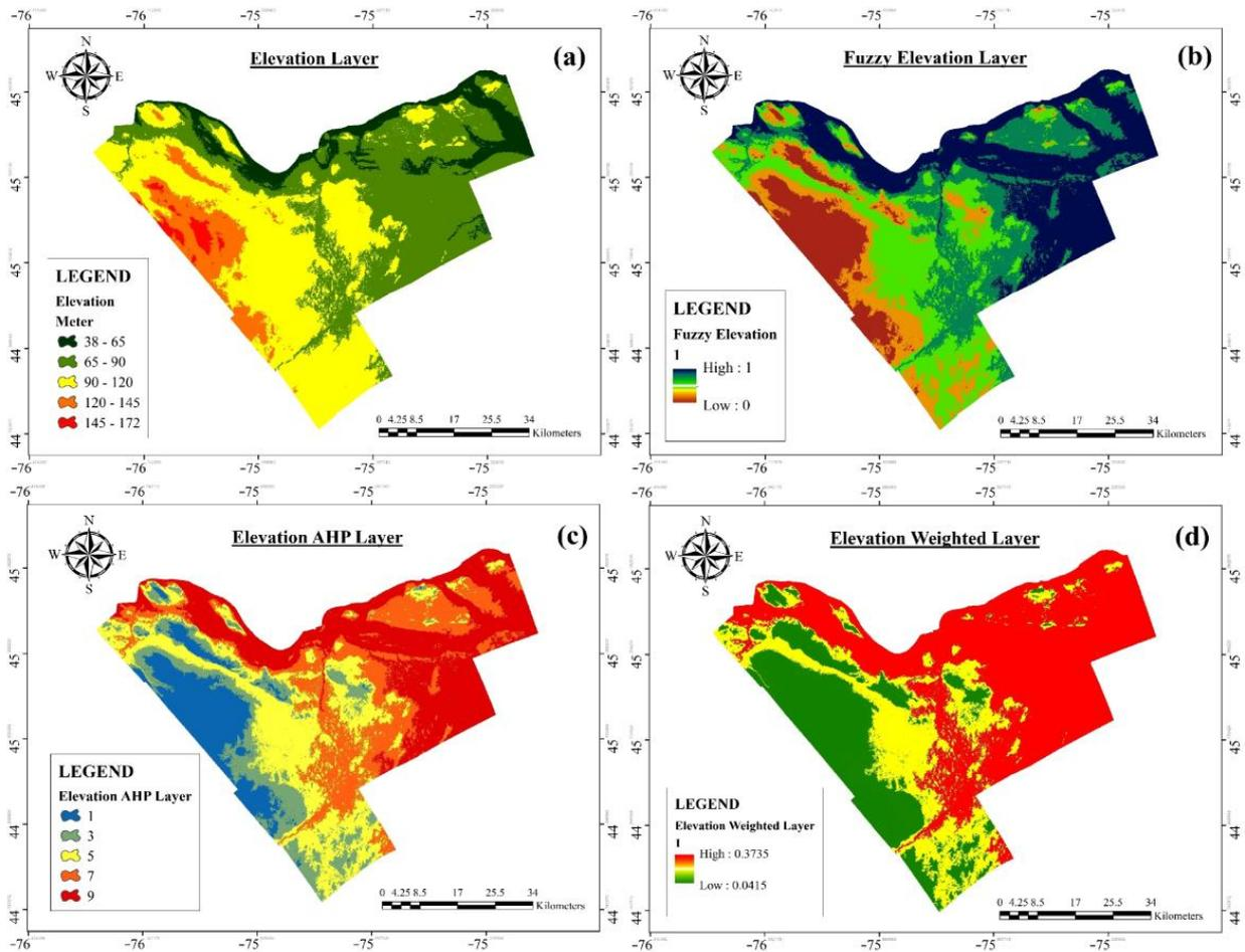
**Figure 3.** The process of fuzzy weighted Elevation layer within a hierarchical GIS model: (a) Elevation raster layer, (b) Fuzzy Elevation layer, (c) Reclassified AHP layer, (d) Weighted Elevation layer.
