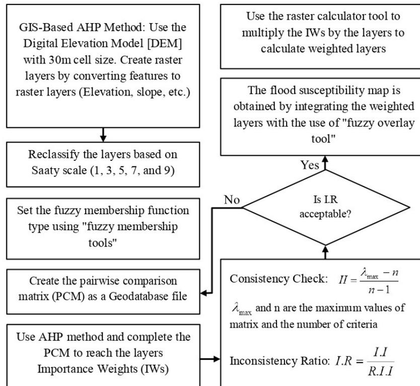
Figure 2. The arrangement of the GIS-based hierarchical model.
