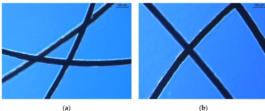
**Figure 2.** Example of the obtained fibers' morphology before (a) and after (b) EOs loading.
