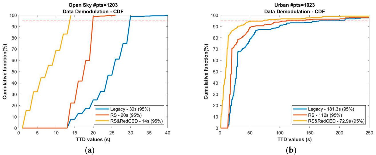
**Figure 3.** Comparison of legacy I/NAV to RS (I/NAV 17–20) and RedCED (I/NAV 16) Data Demodulation: (a) Open Sky CDF of Data Demodulation and (b) Urban CDF of Data Demodulation.
