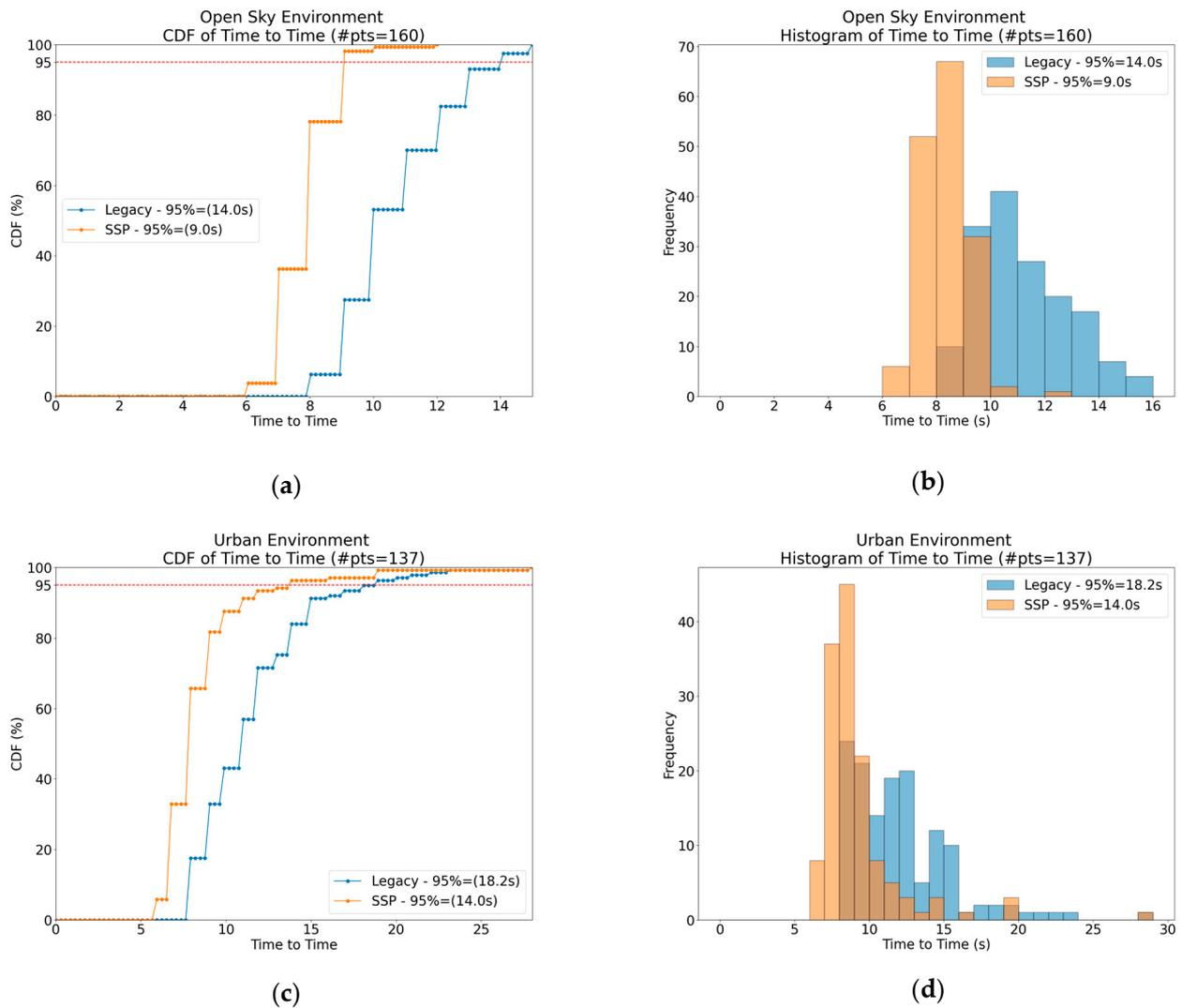
**Figure 4.** Comparison of legacy I/NAV to SSP time-to-time convergence: (a) Open Sky CDF, (b) Open Sky histogram, (c) Urban CDF, (d) Urban histogram.
