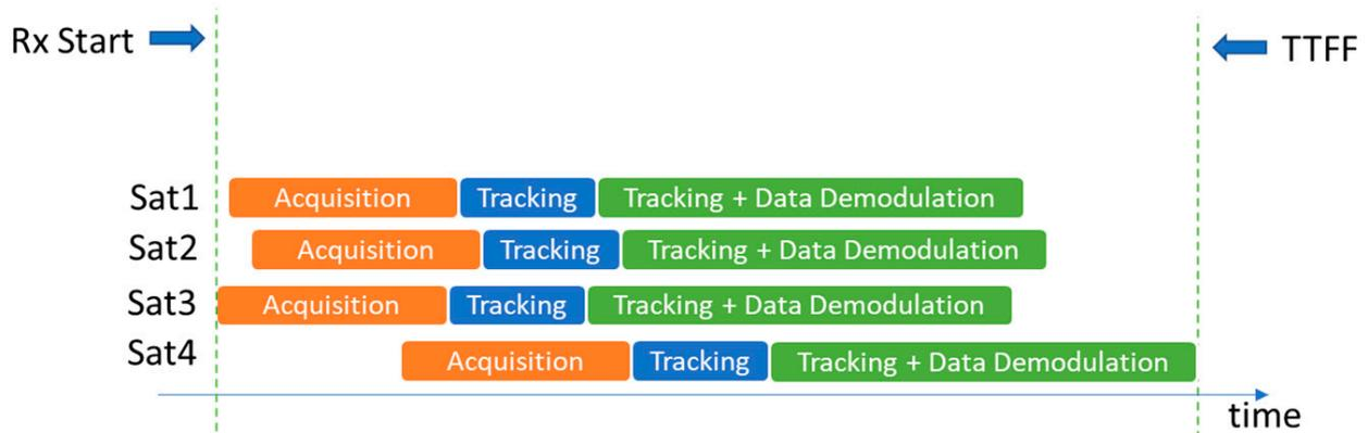
**Figure 2.** Data Demodulation and TTFF visual scheme.
