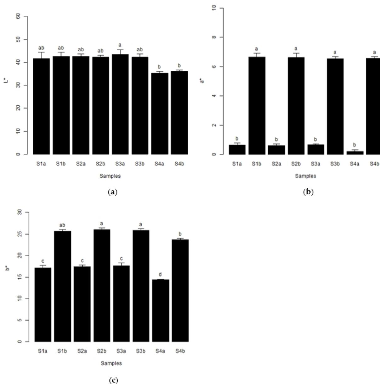
**Figure 1.** Colorimeter CIELab System with the color parameters ( $n = 9$ ): (a)  $L^*$  (lightness); (b)  $a^*$  (red–green transitions); and (c)  $b^*$  (yellow–blue transitions) of soil samples before (S1a, S2a, S3a, and S4a) and after (S1b, S2b, S3b, and S4b) performing organic matter content. Letters a, b, c, d indicate significant differences of each parameter, considering different samples (statistical analysis using the single-factor ANOVA test,  $p < 0.05$ ).
