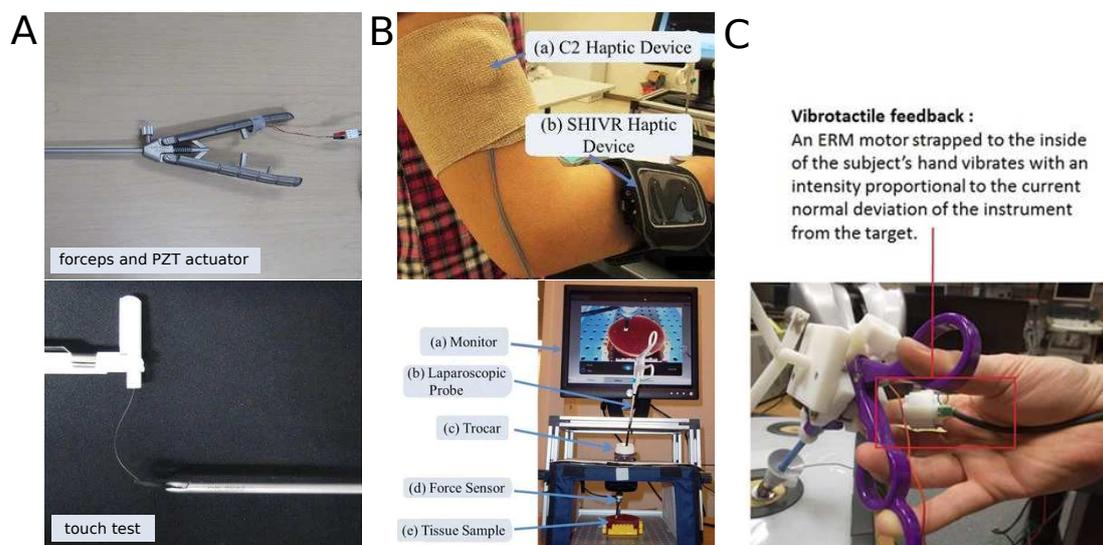
**Figure 4.** Vibrotactile devices. (A) stochastic resonance for laparoscopic surgical instruments [21]; (B) combination of vibrotactile (upper arm) and stochastic resonance (forearm) stimulations for lump detection [22]; (C) vibrotactile feedback for tool guidance [25].
