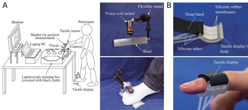
**Figure 5.** Skin indentation devices. (A) rigid factor applies normal force to the foot [28]; (B) pneumatic ring proposed by Ly et al. [30].
