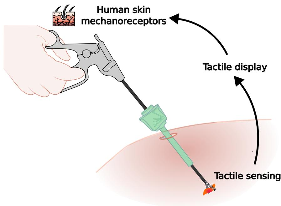
**Figure 1.** Tactile feedback in minimally invasive surgery. Tactile sensors convert the tactile stimuli into data sent to the tactile display, which recreate the same feedback sensation into the human skin mechanoreceptors.
