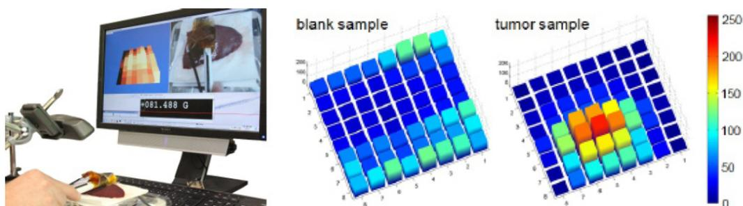
**Figure 6.** Pressure and force represented as a 3D color coded grid and bar graphs [34].
