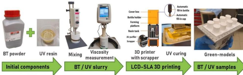
**Figure 5.** Liquid Crystal Display (LCD)-SLA 3D printing of barium titanate ( $BaTiO_3$ )-UV Resin samples [39].
