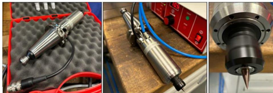
**Figure 3.** Detailed view of the attachment, wiring, and clamped microtool.
