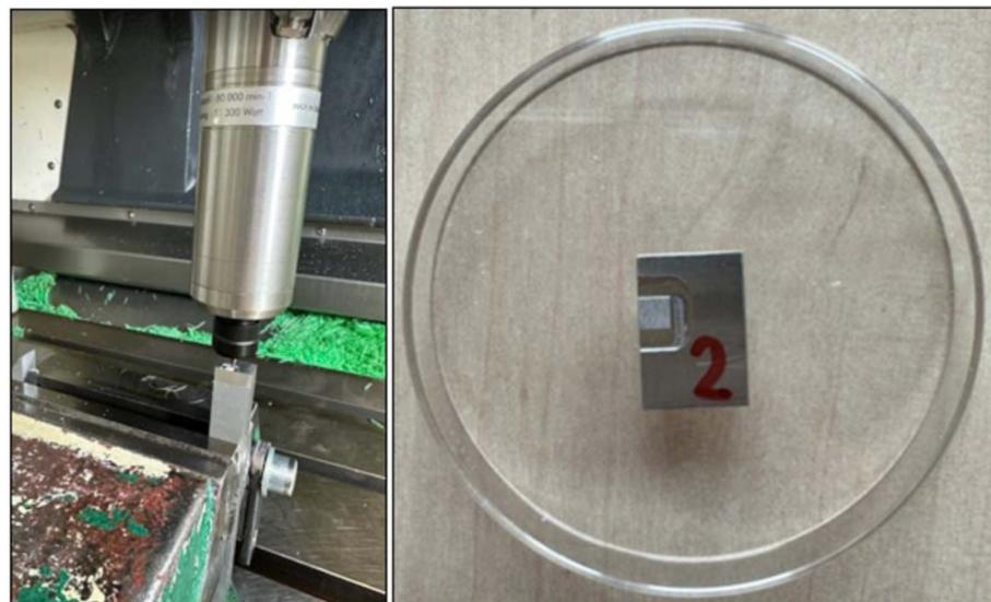
**Figure 8.** Micro-milling process and machined sample with the microstructure.
