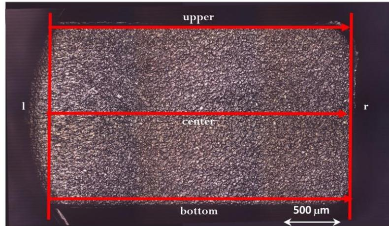
**Figure 3.** Length measurements along three lines parallel to the melt flow (**upper**, **center**, and **bottom**).
