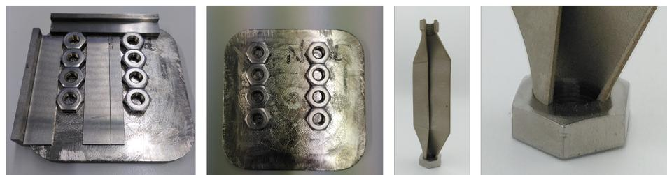
**Figure 4.** Hybrid manufacturing of modules on nuts with an exemplary empty module (three-quarter cut).
