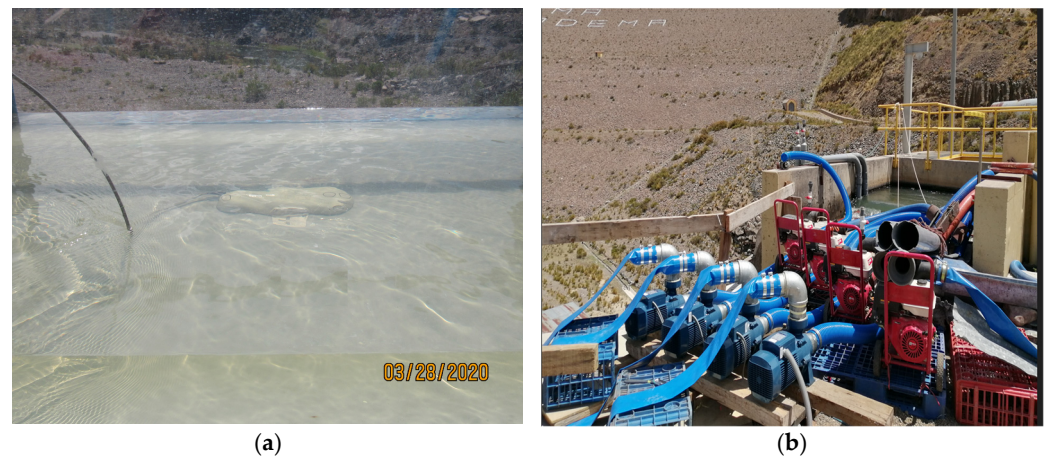
Figure 5. (a) Sontek current meter—IQ plus; (b) pumping system.
