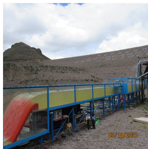
Figure 2. General view of the 21 m long experimental channel located close to Condoroma dam at 4075 m a.s.l.
