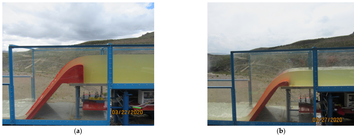
Figure 4. View of two of the ogee-tested profiles: (a) P/H_d = 2 ; (b) P/H_d = 0.5 . Additionally, P/H_d = 1.5, 1 and 0.25 were tested.
