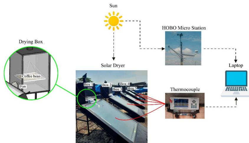
**Figure 3.** Setup of experimental solar collector.
