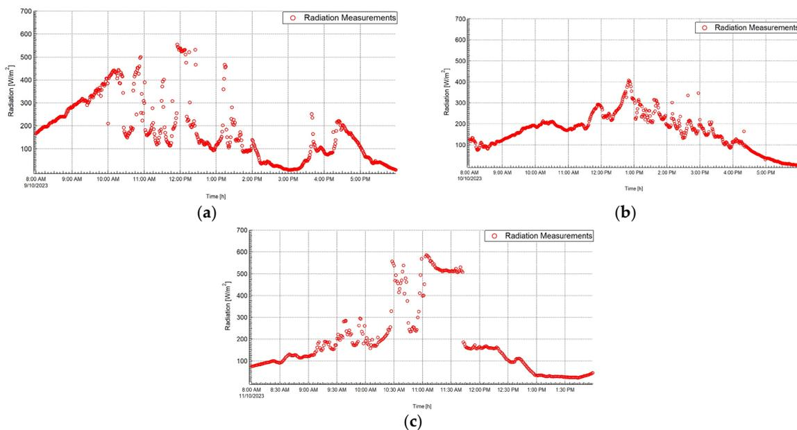
Figure 4. Measured solar radiation: (a) 9 October 2023, (b) 10 October 2023, (c) 11 October 2023.
