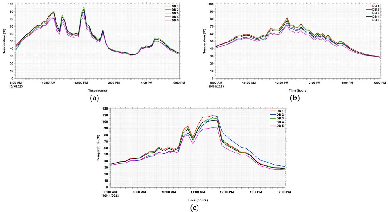
**Figure 6.** Absorbent plate temperature: (a) first day, (b) second day, (c) third day.
