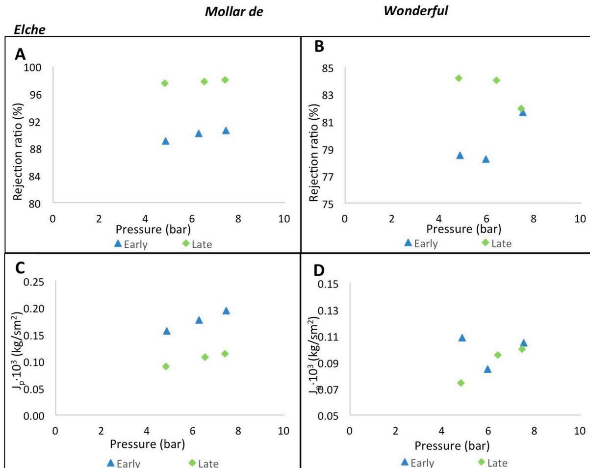
**Figure 3.** Selectivity and efficiency comparison using the rejection coefficient and permeate flux versus pressure, respectively, for *Mollar* (A,C) and *Wonderful* (B,D) varieties at the early and late maturity stage.
