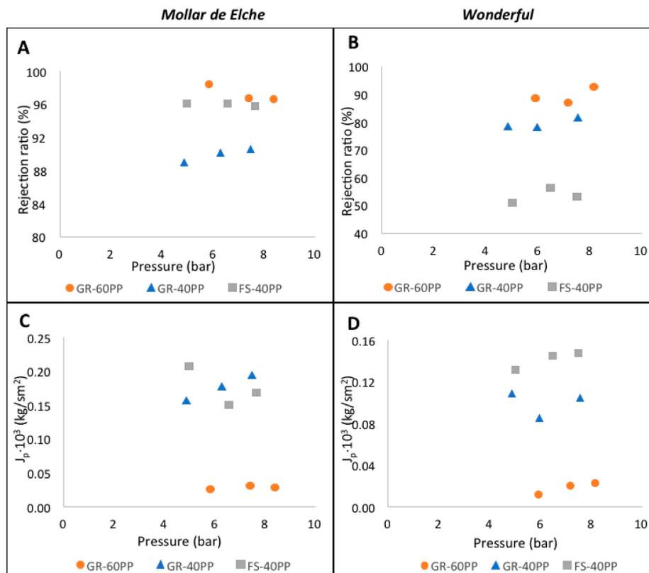
**Figure 2.** Comparison of selectivity and efficiency, using the rejection coefficient and permeate flux versus pressure, respectively, for *Mollar* (A,C) and *Wonderful* (B,D) varieties.
