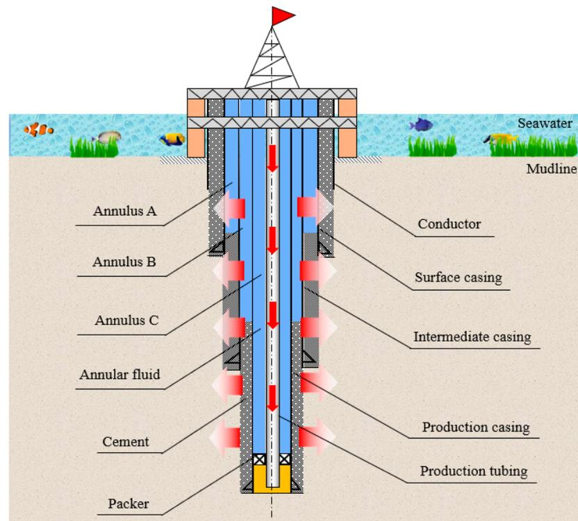
**Figure 1.** The conventional wellbore structure of offshore wells.
