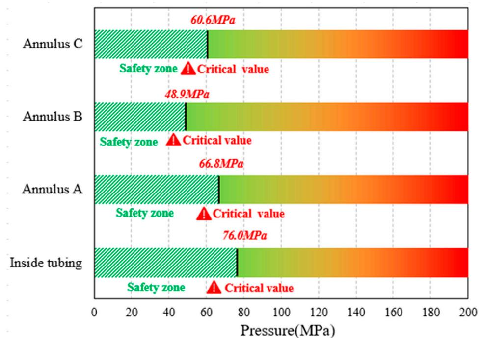
Figure 8. The recommended optimal range of annular pressure.
