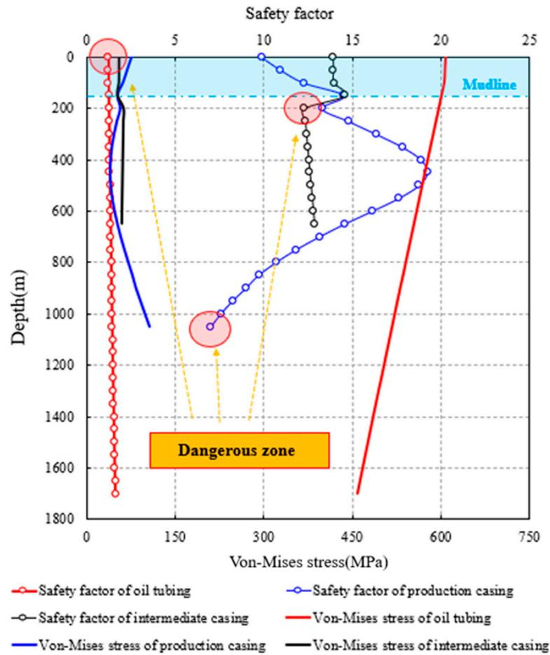
Figure 10. The safety evaluation results of tubing and casing with nitrogen in annulus A.
