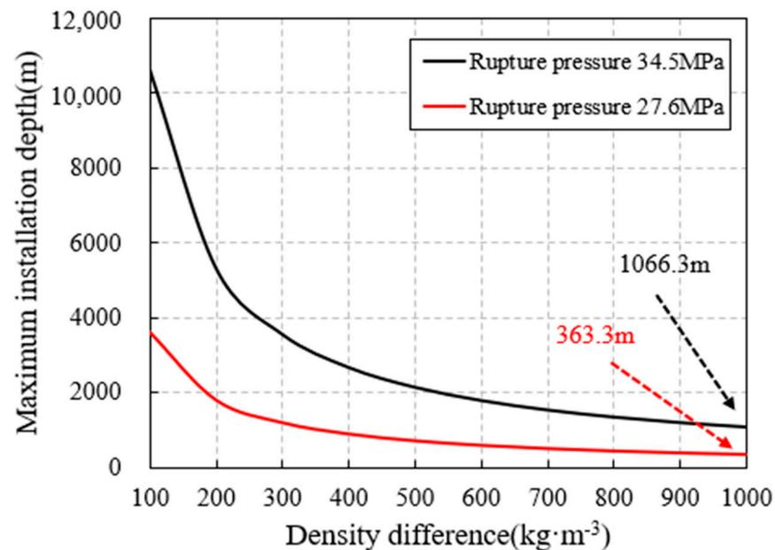
**Figure 13.** The maximum installation depth of rupture disk.
