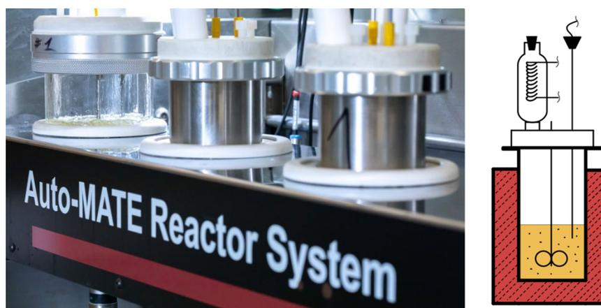
**Figure 6.** The ideal mixing reactor used for synthesis (Auto-MATE Reactor System H.E.L.).
