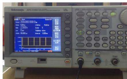
Figure 1. Arbitrary waveform generator for experiment.
