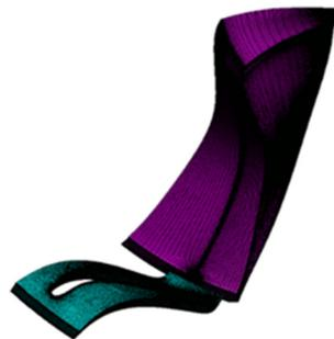
(b) Mesh of nozzle and rotor.
