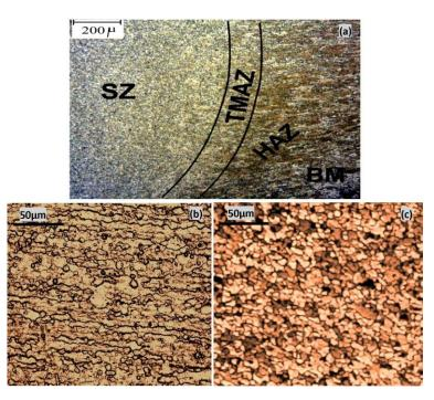
**Figure 8.** Microstructure of the grain distribution in the cross-section of the AA1100 FSW weld (processed at 1120 rpm and 250 mm/min); (**a**) general view of the cross-section, (**b**) stir zone (SZ), and (**c**) the base metal at higher magnification.
