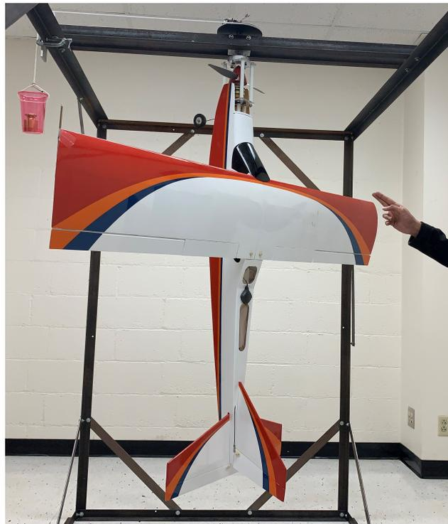
**Figure 9.** Roll moment of inertia testing of the flight-ready Avistar UAV testbed.
