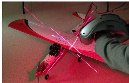
**Figure 6.** The 3D scanning of the Avistar UAV with the ZScanner 800.
