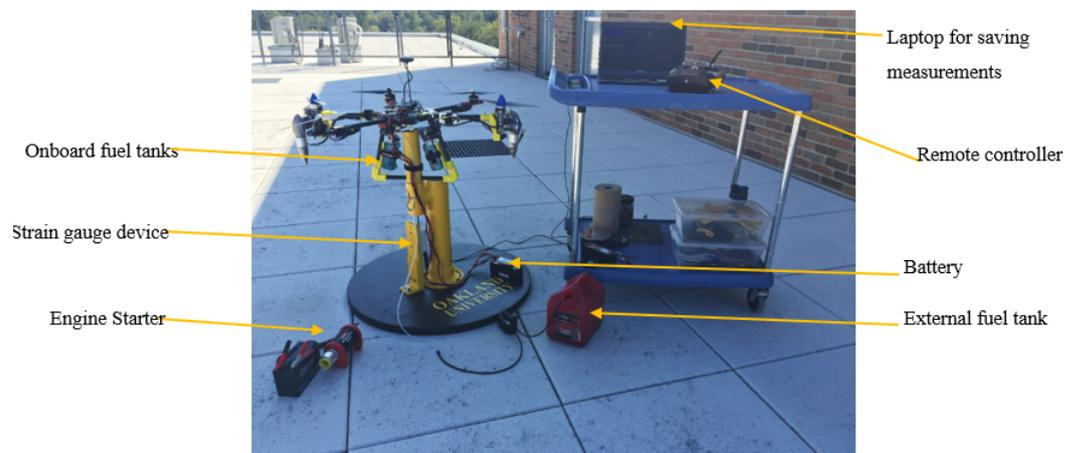
**Figure 21.** Equipment used in controlled experimental testing. The test stand enforced ideal hovering conditions.
