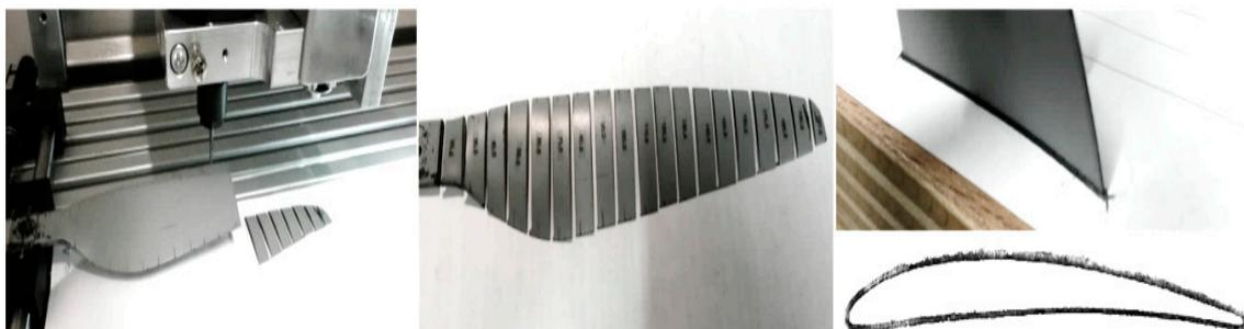
**Figure 5.** Rotor airfoil tracing method. Cuts obtained at various rotor span stations using a CNC mill.
