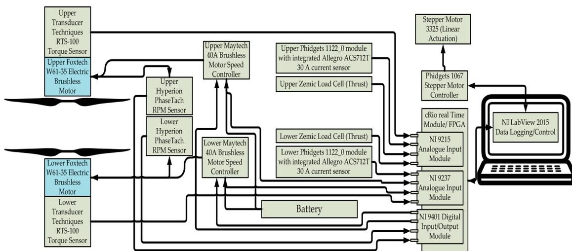
**Figure 9.** Test rig system diagram.
