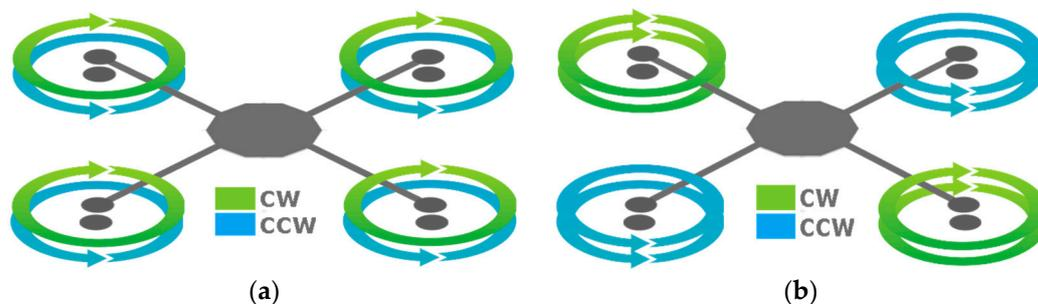
**Figure 1.** Overlapping rotor propulsion system co-axial quadrotor configurations: (a) system torque balanced at all four propulsion units internally; and (b) system torque balance achieved externally of the individual propulsion units.
