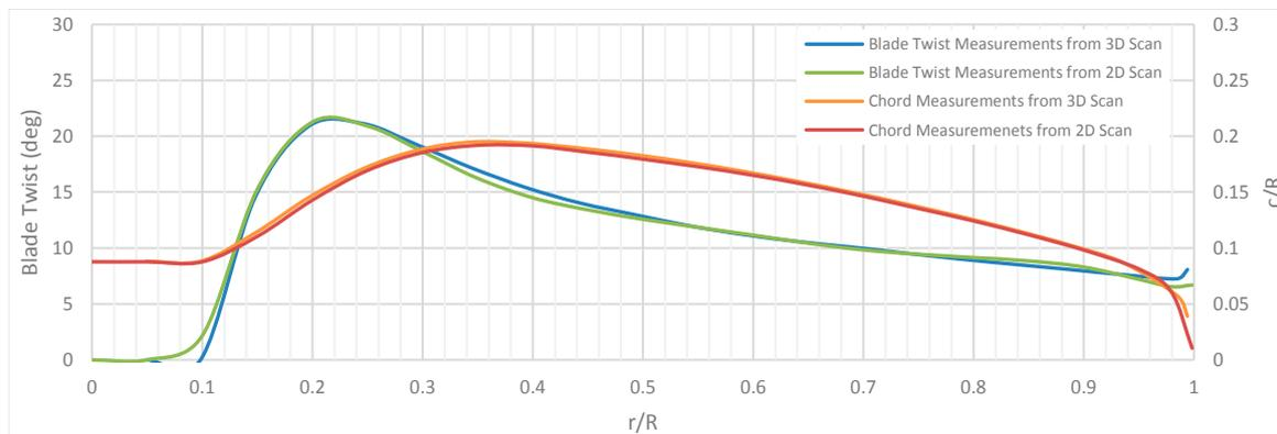
**Figure 6.** T-Motor 16 inch  $\times$  5.4 inch blade twist and chord length at various rotor blade span stations  $r/R$ .
