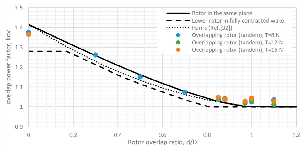
**Figure 20.** Overlapping rotor (tandem)-induced power correction  $k_{ov}$  for the hover state, derived from momentum theory ( $z/D = 0.05$ ).
