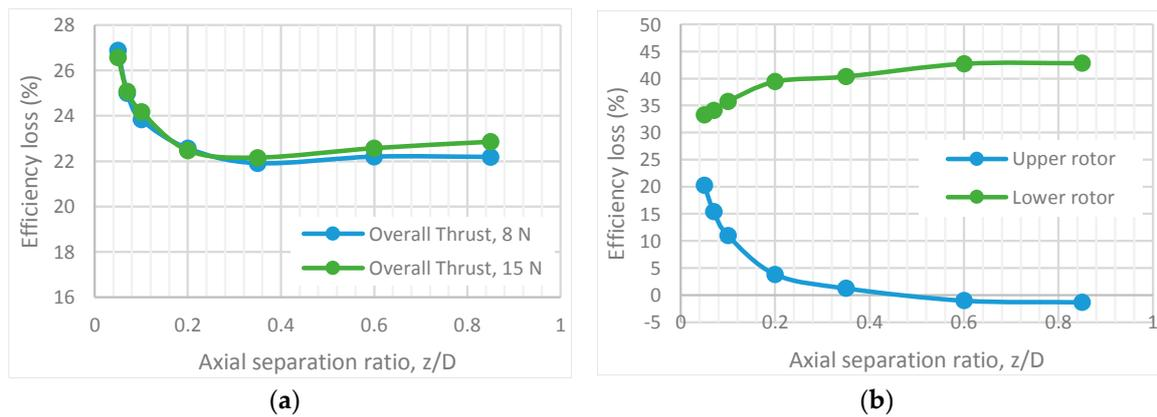
**Figure 15.** Co-axial propulsion system efficiency losses at various  $z/D$  ratios. (a) Overall co-axial system efficiency losses ( $Q_u + Q_l = 0$ ); (b) Individual rotor efficiency losses when operated in a co-axial setup ( $Q_u + Q_l = 0$ ); overall thrust, 8 N.
