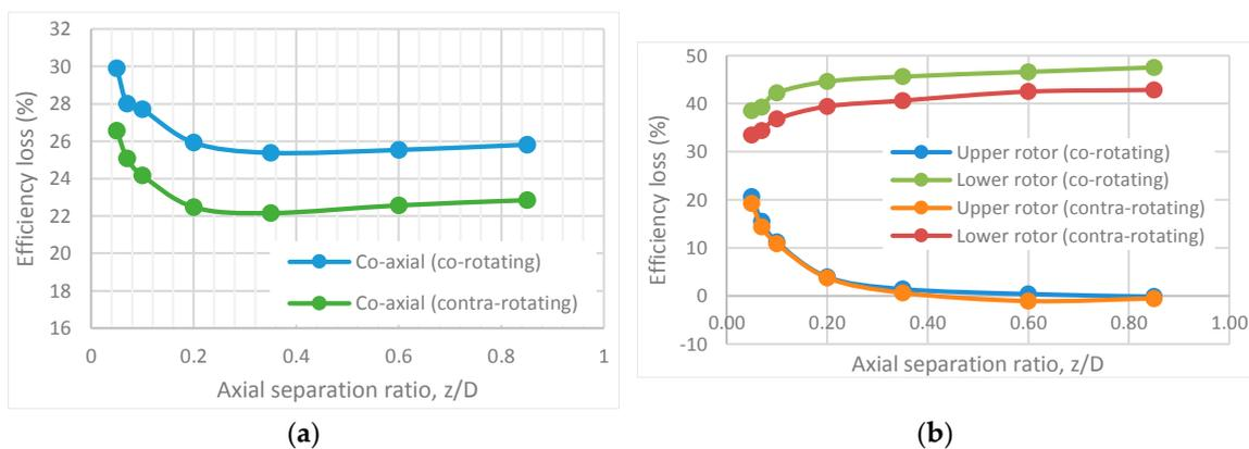
**Figure 16.** Performance comparison quantifying losses/gains of co-rotating rotor co-axial and conventional co-axial setups over two isolated rotors (overall thrust, 15 N). (a) Co-axial system performance; (b) Individual rotor performance.
