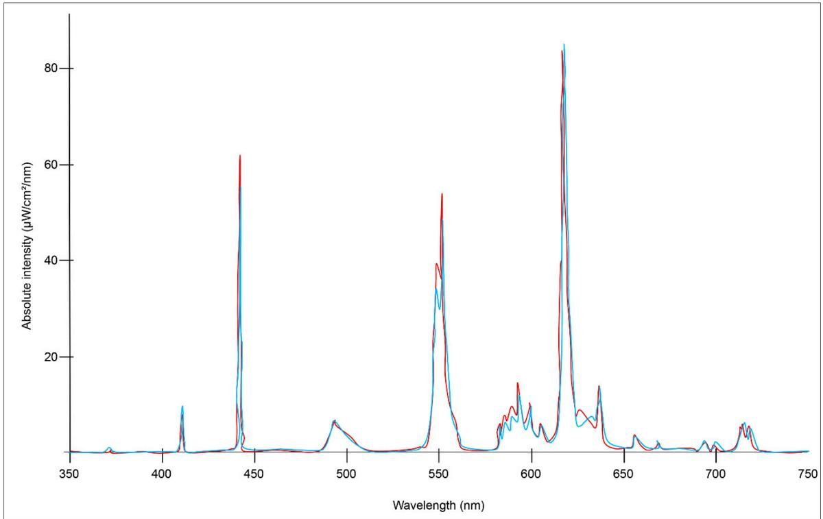
Figure S1: Comparison of the spectral output of a new fluorescent lamp (blue line) with one approximately six months old (red line).
