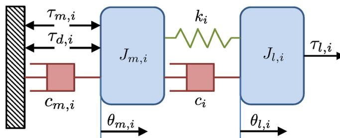
Figure 6. The two-mass model selected for each joint.
