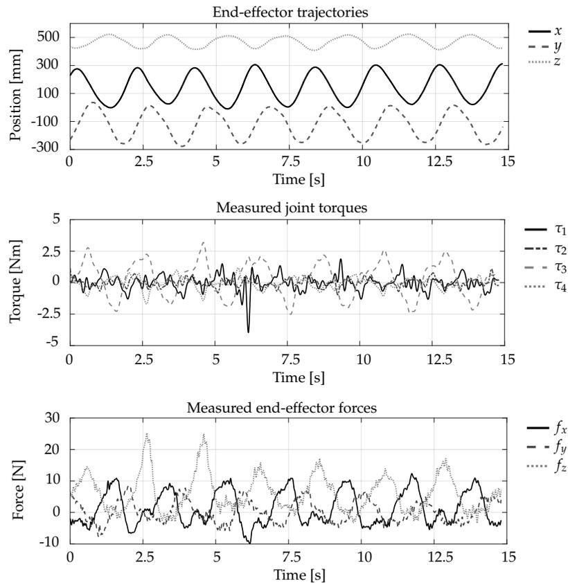
**Figure 15.** Results of the transparency test with the JTFC1 controller. The user can perform circular trajectories in the XY plane at constant speed (first row). On the second row, the residual joint torques are reported. The controlled joints exhibit a good transparency, as highlighted by the limited value of the residual torque compared to the maximum exertable one. The plot on the third row reports the interaction forces measured at the end effector, always smaller than 25 N.
