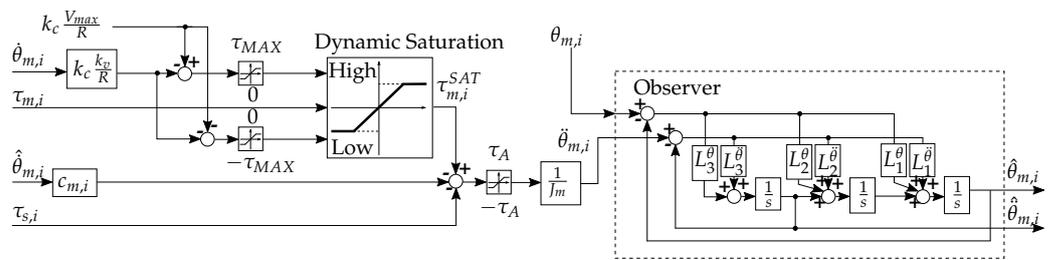
**Figure 8.** Block scheme of the acceleration estimator basing on torque measurements. The left side of the scheme models the motor dynamics, and it takes into account saturation effects. The right side of the scheme shows the implementation of the observer.
