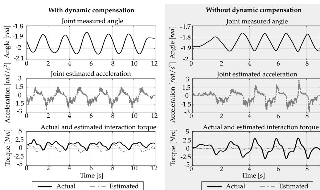
**Figure 11.** Comparison between the two experiment conditions: w. (left) and w.o. dynamic compensation (right, in gray). The three sets of rows show, respectively, the measured angular position of the joint, its estimated acceleration and a comparison between actual and estimated joint torque. The latter is computed by the force sensor for the joint  $J_2$ . Without dynamics compensations, the actual torques differ from the estimated ones, resulting in a loss of transparency.
