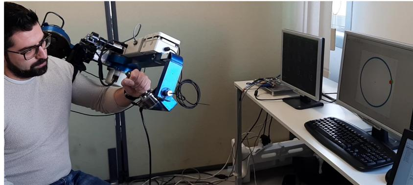
**Figure 12.** Experimental setup for the transparency test. The user is connected to the exoskeleton at shoulder level and at the end effector, grabbing the handle. The user’s elbow and the exoskeleton’s one are in contact during the trial execution. The subject moves the exoskeleton, performing a circular trajectory at a constant angular speed, whose reference is displayed on a screen.
