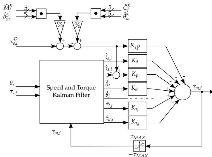
**Figure 10.** Schema of the full-state feedback controller that implements the dynamic compensation. Inertial and Coriolis effects make use of the estimated joint accelerations and velocities (see scheme of Figure 8).
