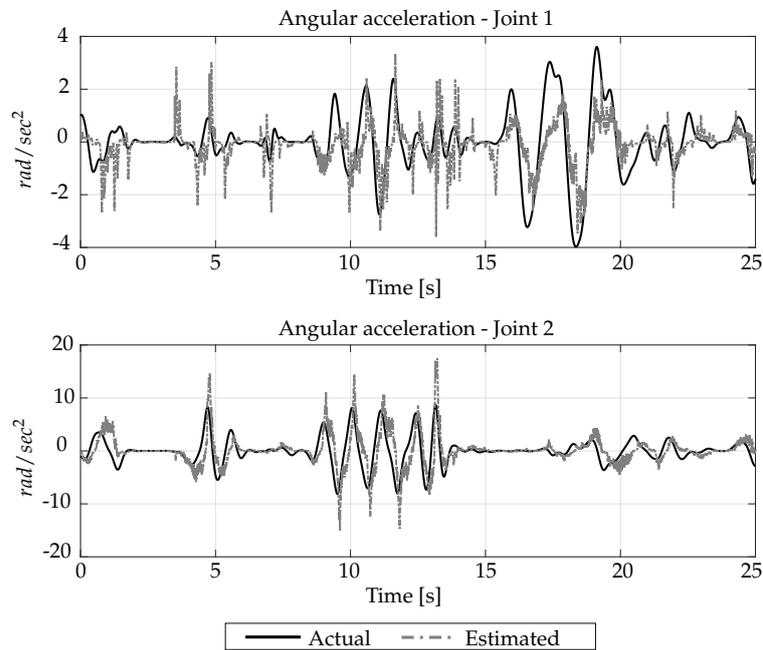
**Figure 9.** Comparison between estimated (gray dashed line) and actual (solid black line) joint acceleration. Joints  $J_1$  and  $J_2$  are chosen for reference only. Similar results are obtained for all the joints.
