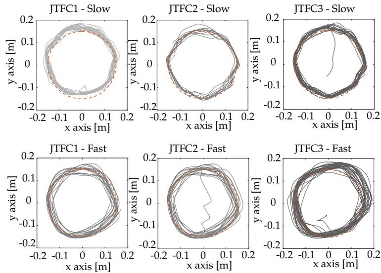
**Figure 14.** The trajectories performed during the transparency test using the three control laws in the slow-speed (first row) and fast-speed (second row) conditions. The red dashed lines are the circular reference trajectories.
