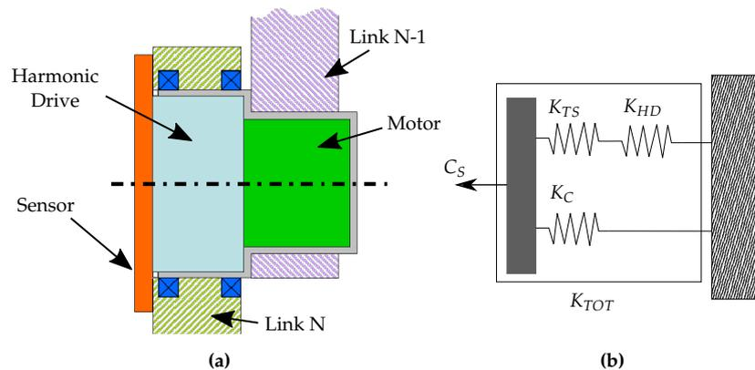
**Figure 5.** (a) Schematic view of the joint. The torque sensor connects in series the motor and the link  $n$ ; nevertheless, it is not structural and is designed to transmit only axial torque. (b) The kinematic chain of the joint to non-axial loads.  $K_{TS}$  and  $K_{HD}$  represent the stiffness of the torque sensor and of the harmonic drive to non-axial load, respectively, whereas  $K_B$  is the bearing stiffness.
