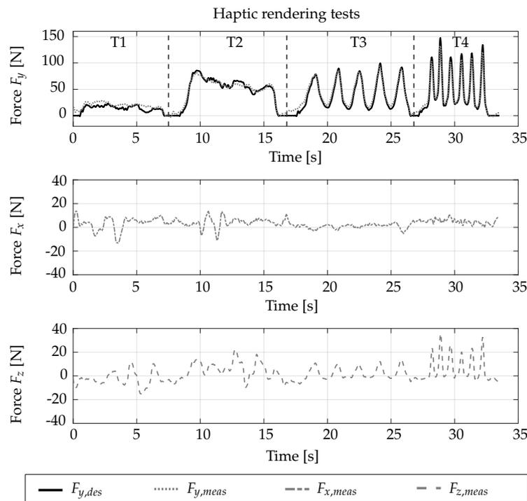
**Figure 16.** The four trials of the whole haptic rendering test. The desired forces  $F_{y,des}$  are plotted with a black solid line, whereas the measured orthogonal forces  $F_{y,meas}$  are plotted with a gray dotted line in the first row. The two tangential components  $F_{x,meas}$  and  $F_{z,meas}$  are shown in the second and third rows, respectively.
