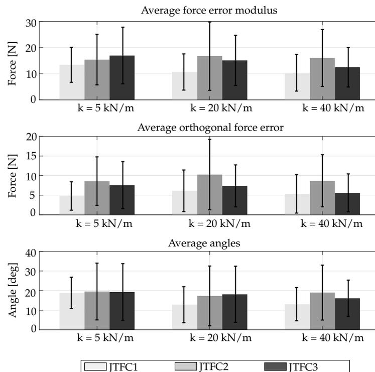
**Figure 17.** The first row shows the average of the modulus of the error force vectors at the end effector of the three controllers in the rendering task. For this test, three stiffnesses are evaluated: 5 kN/m (small), 20 kN/m (medium) and 40 kN/m (high). The second row shows the average error forces of the orthogonal component. The third row shows the average angle between the desired force vectors and the measured ones.
