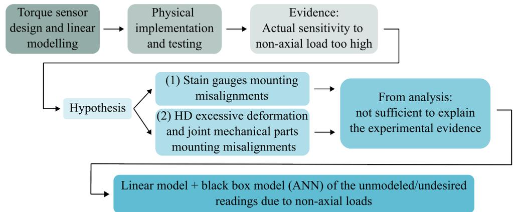
**Figure 4.** Roadmap of the analysis conducted on the sensitivity to non-axial load of the torque sensor.
