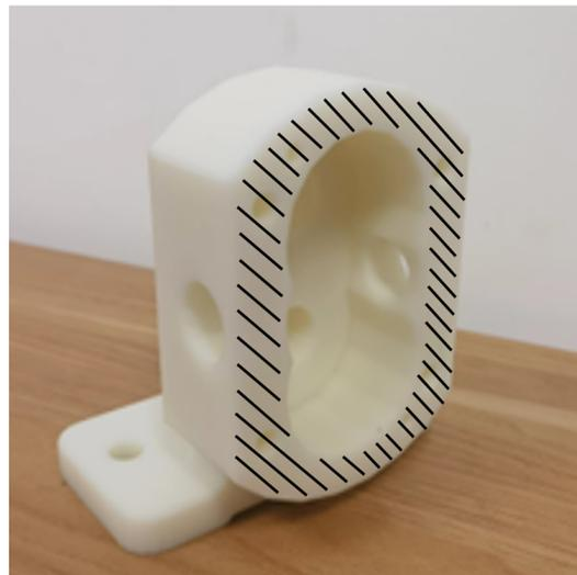
**Figure 3.** The workpiece, a gear pump housing, a mock-up made of resin material.
