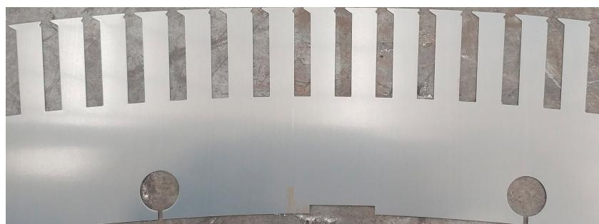
**Figure 3.** Stator slots of the LHPMSM.
