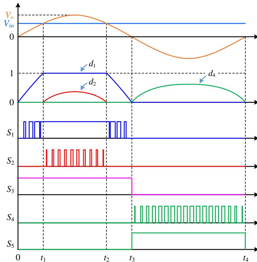
Figure 2. PWM control method of the proposed CGBBI topology.
