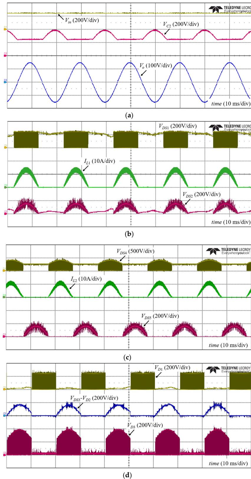
**Figure 9.** Experimental results with  $V_{in} = 240$  V. (a) the input, output and capacitor  $C_2$  voltages, (b) the voltage stress on switches  $S_1, S_2$ , and the current of inductor  $L_1$ , (c) the voltage stress on switches  $S_4, S_5$ , and the current of inductor  $L_2$ , and (d) the voltage stress on diodes  $D_1, D_2, D_3$  and the voltage stress on switch  $S_3$ .
