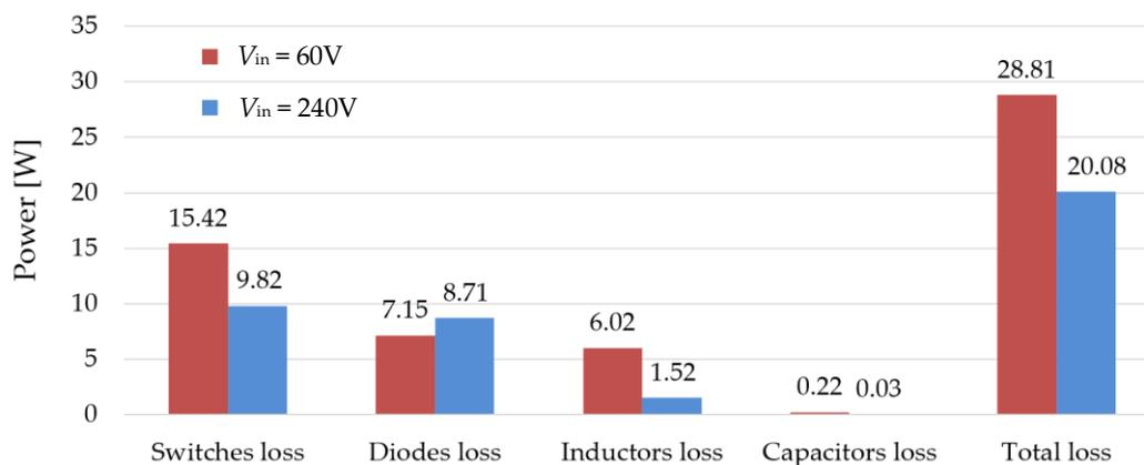
Figure 11. Power loss distribution of the proposed CGBBI.
