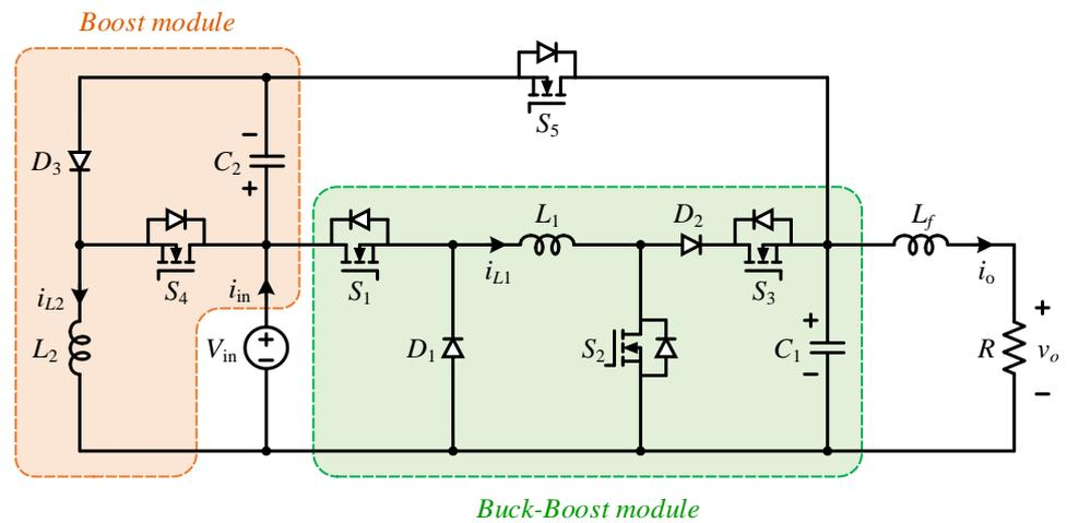
Figure 1. Proposed single-stage common-ground buck-boost inverter.
