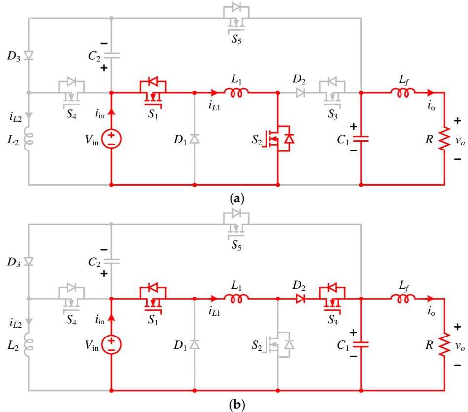
**Figure 4.** Equivalent circuits of the proposed CGBBI topology in interval 2 when  $v_o > V_{in}$ : (a) mode 1 and (b) mode 2.
