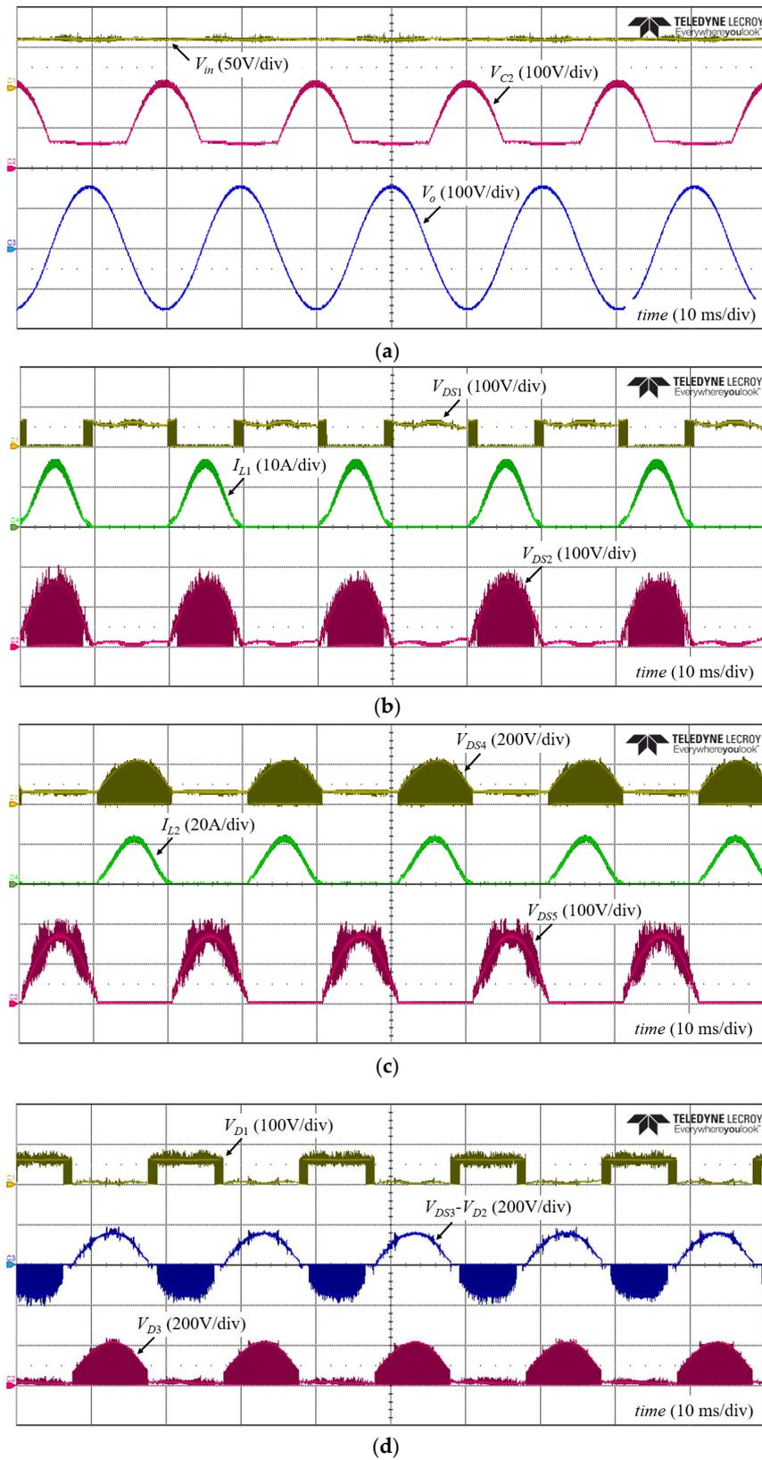
**Figure 8.** Experimental results with  $V_{in} = 60$  V. (a) the input, output and capacitor  $C_2$  voltages, (b) the voltage stress on switches  $S_1, S_2$ , and the current of inductor  $L_1$ , (c) the voltage stress on switches  $S_4, S_5$ , and the current of inductor  $L_2$ , and (d) the voltage stress on diodes  $D_1, D_2, D_3$  and the voltage stress on switch  $S_3$ .
