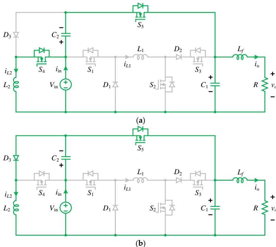
Figure 5. Equivalent circuits of the proposed CGBBI topology in interval 3 when  $v_o < 0$ : (a) mode 1 and (b) mode 2.
