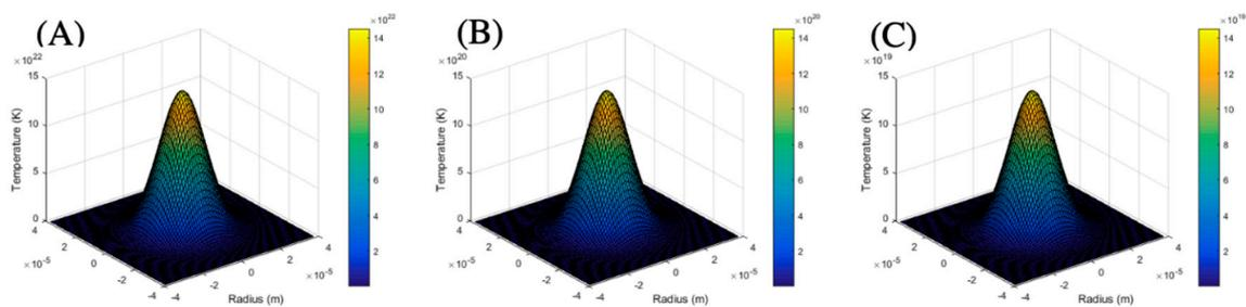
**Figure 5.** The 3D temperature gradient profile for (A) laser frequency of 600 kHz; (B) laser frequency of 800 kHz; and (C) laser frequency of 1200 kHz.
