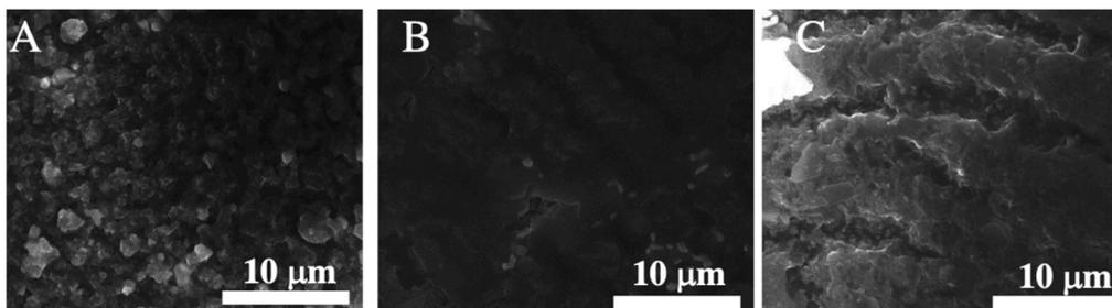
**Figure 8.** SEM images of samples after immersion in SBF solution. (A) Produced by laser frequency of 600 kHz and immersed in SBF for 4 days; (B) produced by laser frequency of 800 kHz and immersed in SBF for 4 days and (C) produced by laser frequency of 1200 kHz and immersed in SBF for 4 days.
