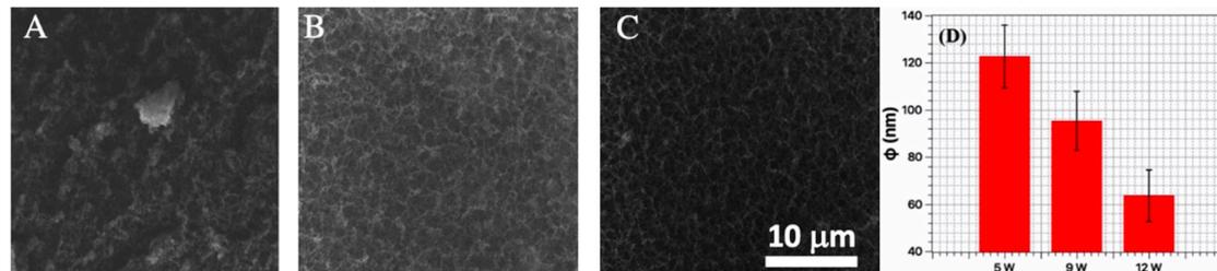
**Figure 1.** Scanning electron microscope (SEM) images of (A) nanofibrous titanium (NFTi) deposited layer on glass with laser power of 5 W; (B) NFTi deposited layer on glass with laser power of 9 W; and (C) NFTi deposited layer on glass with laser power of 12 W; (D) Column chart of fiber diameters by increased laser power.
