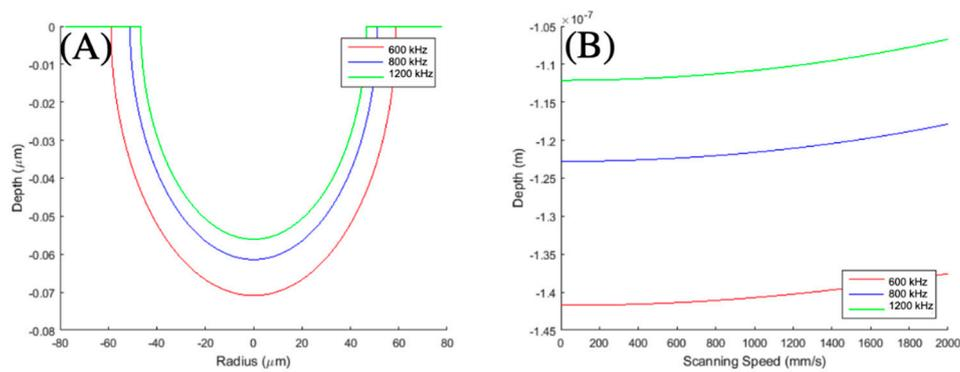
**Figure 6.** (A) Theoretical ablation depth profile as a function of radius and (B) theoretical ablation depth profile as a function of laser scanning speed for single pulsed laser with frequency of 600, 800 and 1200 kHz.
