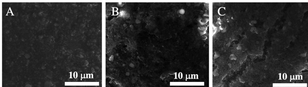
**Figure 7.** SEM images of samples after immersion in simulated body fluid (SBF) solution. (A) Produced by laser power of 5 W and immersed in SBF for 4 days; (B) produced by laser power of 9 W and immersed in SBF for 4 days and (C) produced by laser power of 12 W and immersed in SBF for 4 days.
