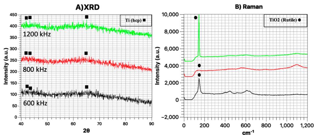
**Figure 11.** (A) XRD pattern and (B) Raman spectrum of glass samples coated by titanium with different laser frequencies.
