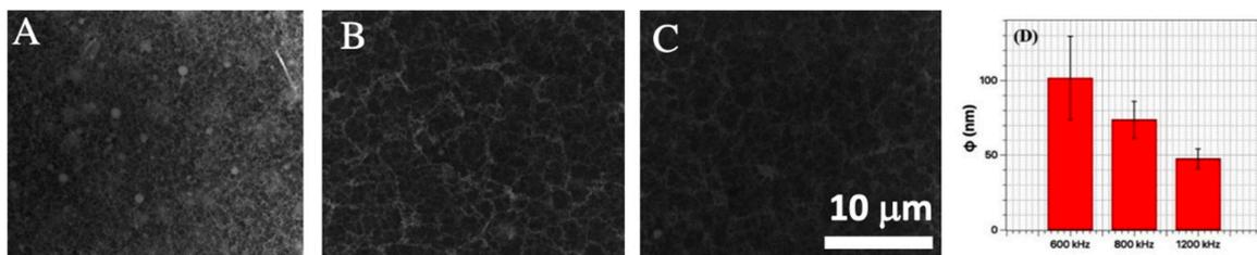
**Figure 4.** SEM images of (A) NFTi deposited layer on glass with laser frequency of 600 kHz; (B) NFTi deposited layer on glass with laser frequency of 800 kHz and (C) NFTi deposited layer on glass with laser frequency of 1200 kHz; (D) Column chart of fiber diameters by increasing laser frequency.
