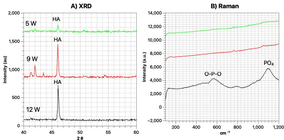
**Figure 10.** (A) XRD pattern and (B) Raman spectrum of glass samples coated by titanium with different laser powers after 4 days immersion in SBF.
