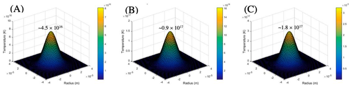
**Figure 2.** The 3D radial temperature gradient profiles for laser power of (A) 5 W; (B) 9 W and (C) 12 W.
