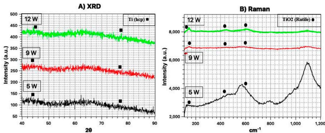
**Figure 9.** (A) X-ray diffraction (XRD) pattern and (B) Raman spectrum of glass samples coated by titanium with different laser powers.
