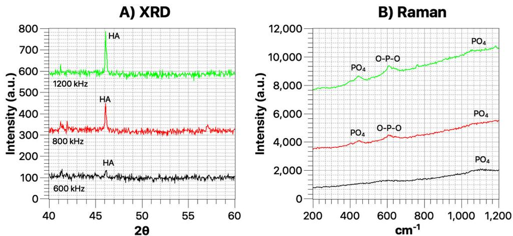
**Figure 12.** (A) XRD pattern and (B) Raman spectrum of glass samples coated by titanium with different laser frequencies after 4 days immersion in SBF.
