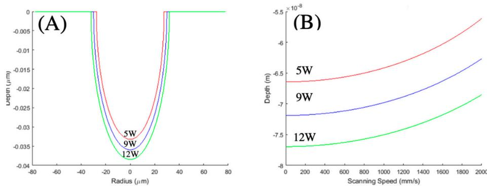
**Figure 3.** (A) Theoretical ablation depth profile as a function of radius and (B) theoretical ablation depth profile as a function of laser scanning speed for single pulsed laser with powers of 5, 9 and 12 W.
