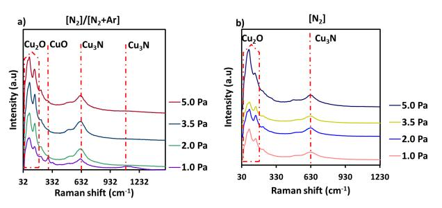
**Figure 5.** Raman spectra for Cu<sub>3</sub>N films deposited at different pressures on glass. (a)  $[N_2]/[N_2 + Ar]$  r = 0.7 and (b)  $[N_2]$  r = 1.0.
