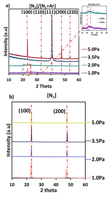
**Figure 3.** X-ray diffraction spectra of  $Cu_3N$  films at different gas pressures (Pa) and nitrogen flow ratios. (a)  $[N_2]/[N_2 + Ar] r = 0.7$  and (b)  $[N_2] r = 1.0$ .
