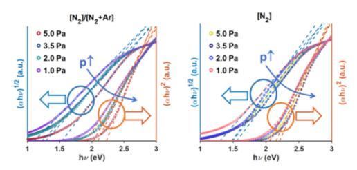
**Figure 8.** A plot of  $(\alpha h\nu)^{1/2}$  and  $(\alpha h\nu)^2$  vs. photon energy (eV) for the Cu<sub>3</sub>N films at different gas pressures and atmospheres. For ease of comparison, normalised values of the absorption coefficient are considered.
