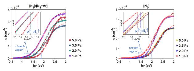
**Figure 9.** Absorption coefficient spectra of  $Cu_3N$  layers at different pressures and atmospheres. The red dashed lines show the fit according to the model equations described (5)–(8). In the logarithmic scale, the insets show the exponential tail of the Urbach region; note the effect of pressure on the transition energy  $E_1$ .
