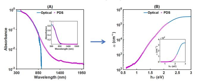
**Figure 7.** Absorbance obtained from optical measurements and PDS for the  $Cu_3N$  film deposited at 5.0 Pa pressure in pure  $N_2$  atmosphere. In (**A**), the absorbance spectra are shown, and in (**B**), the absorption coefficient is calculated from the fit based on the transfer matrix method. The insets show the same graphs on a linear scale.
