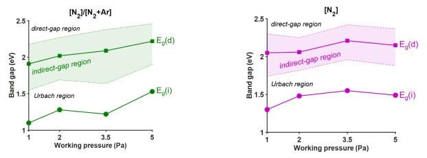
**Figure 10.** Evolution with a working pressure of the energies of the direct gap Eg(d) and the indirect gap Eg(i) for the two deposition atmospheres. The shaded region indicates the range of photon energies ( $E_1 < hv < E_2$ ) associated with electronic transitions according to the indirect gap: for higher energies ( $hv > E_2$ ), the transitions are associated with the direct gap and for lower energies ( $hv < E_1$ ) with the Urbach tail.
