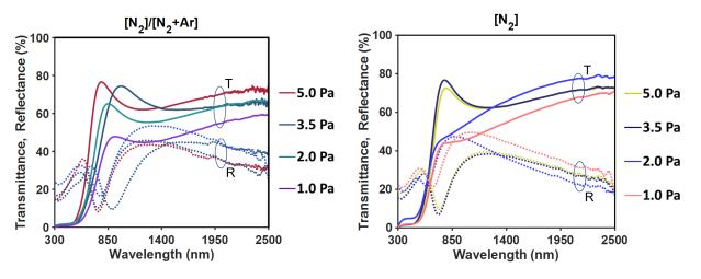
**Figure 6.** Transmittance and reflectance spectra of Cu<sub>3</sub>N films deposited at different pressures and atmospheres.
