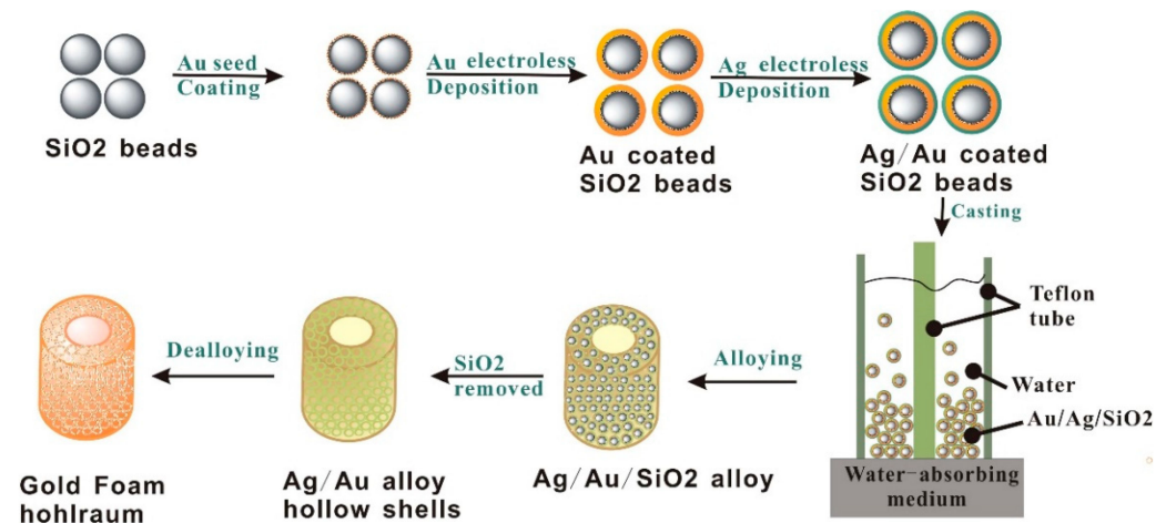
Figure 1. Schematic illustration of Au foam hohlraum fabrication.
