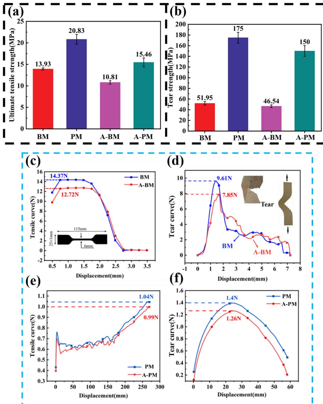
**Figure 6.** (a) Tensile strength of BM paper film and PM white film before and after dry heat aging; (b) tear strength of BM and PM before and after dry heat aging; (c) tensile curve of BM paper film before and after aging; (d) tear curve of BM paper film before and after aging; (e) tensile curve of PM white film before and after aging; (f) tear curve of PM white film before and after aging.
