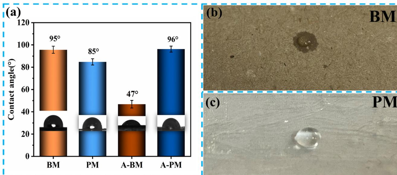
**Figure 7.** (a) Surface contact angle of BM and PM before and after dry heat aging; (b) physical image of BM; (c) physical image of PM.
