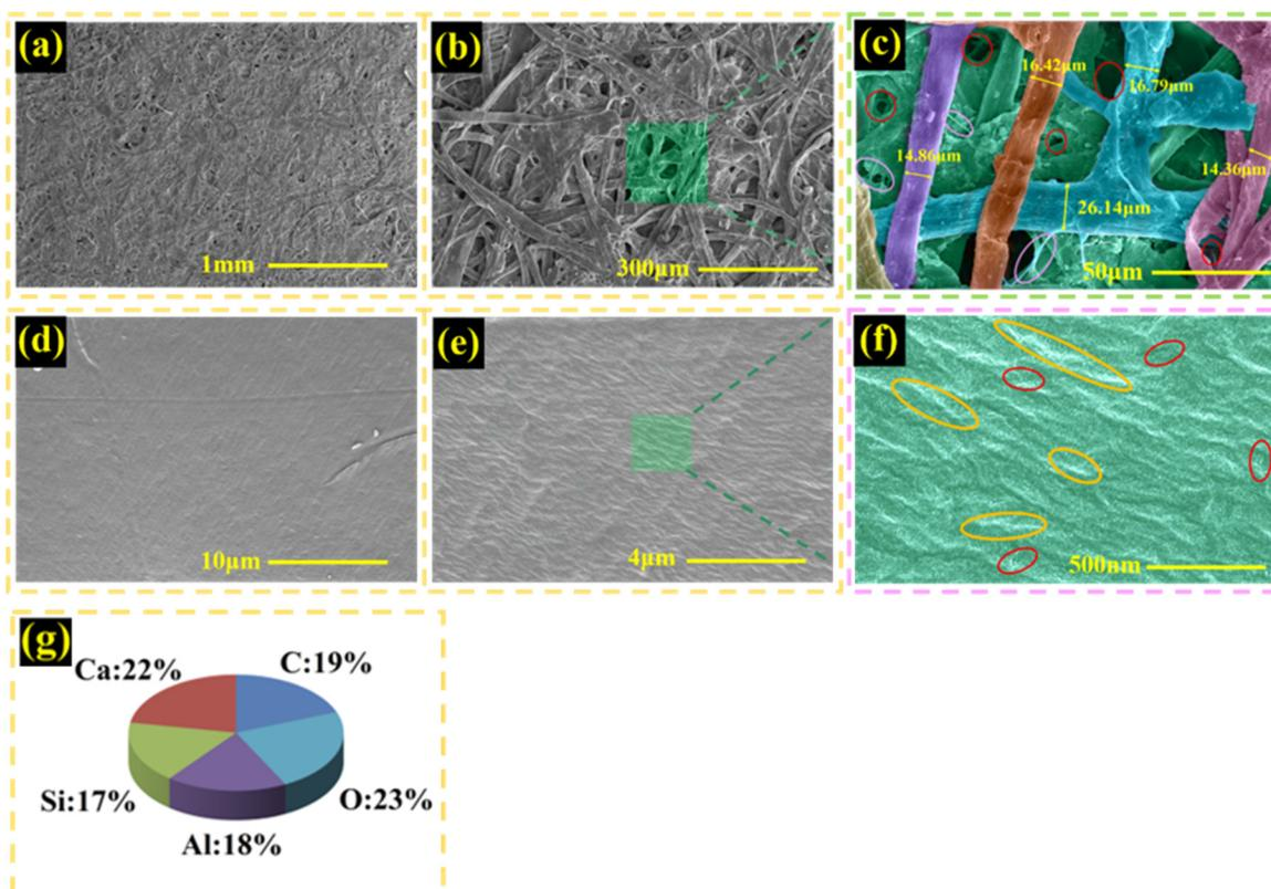
**Figure 5.** (a–c) SEM images of biodegradable paper film surface at different magnification; (d–f) SEM images of plastic white film surface at different magnification; (g) element content distribution on the surface of BM.
