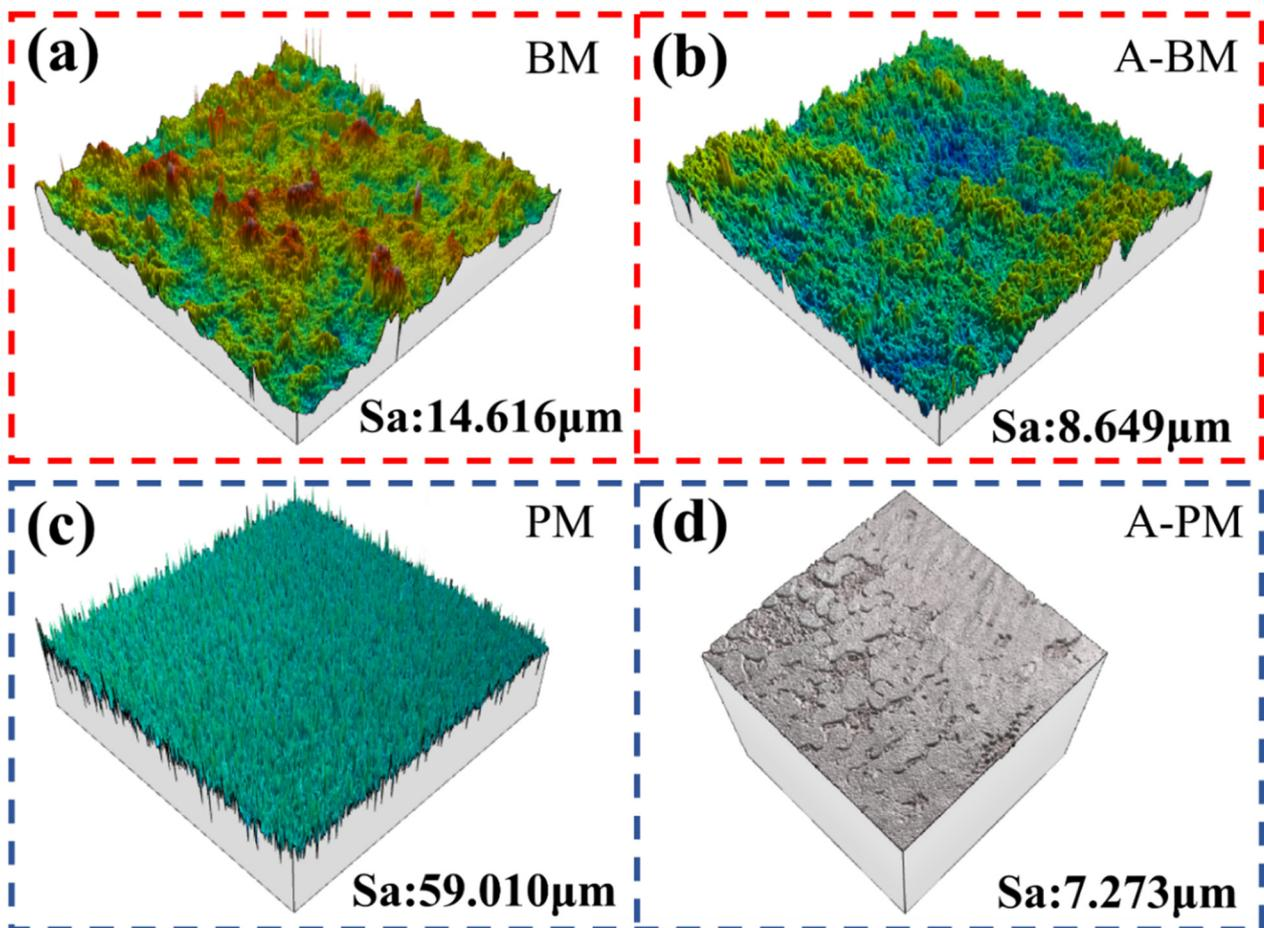
**Figure 8.** Three-dimensional morphology of (a) BM surface, (b) aged BM surface, (c) PM surface, and (d) aged PM surface.
