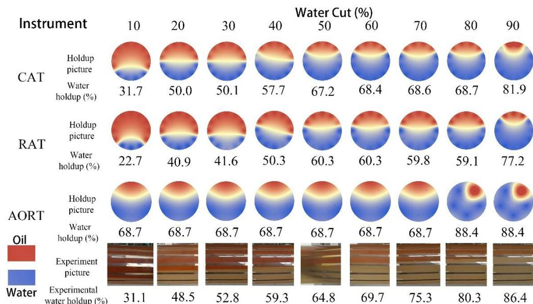
Figure 8. Comparison of interpolation imaging under different water cut conditions of  $30 \text{ m}^3/\text{d}$  of oil and water.
