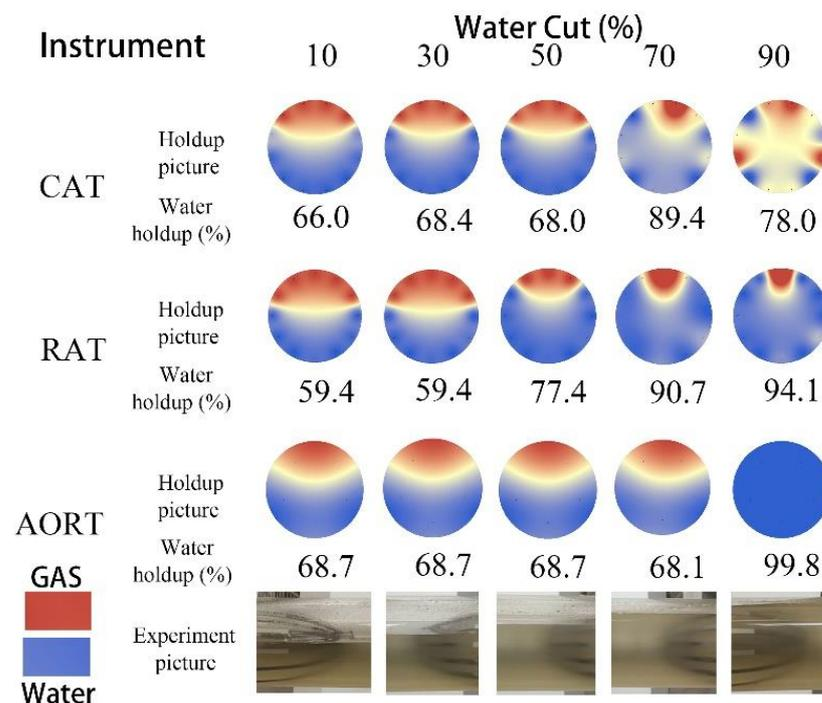
Figure 7. Comparison of interpolation imaging under different water cut conditions of  $300 \text{ m}^3/\text{d}$  of gas and water.
