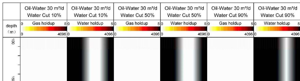
Figure 6. Response characteristics when the water cut of  $30 \text{ m}^3/\text{d}$  of oil and water is 10%, 50%, and 90%.
