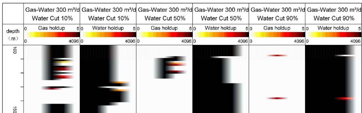
Figure 5. Response characteristics when water cut of  $300 \text{ m}^3/\text{d}$  of gas and water is 10%, 50%, and 90%.
