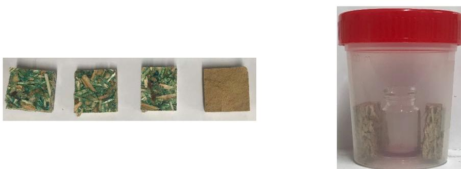
**Figure S10.** Left (different board pieces, from left to right PB 27 mm, PB 10 mm, PB 16 mm, FB 35 mm). Right (system for the detection of the formaldehyde emission from board pieces).
