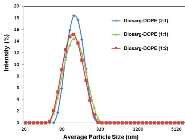
**Figure S2.** Hydrodynamic average particle sizes of the Diosarg-1,2-dioleoyl-sn-glycero-3-phosphoethanolamine (DOPE) (2:1, 1:1, 1:2) NPs in distilled water at room temperature measured by the dynamic light scattering instrument.
