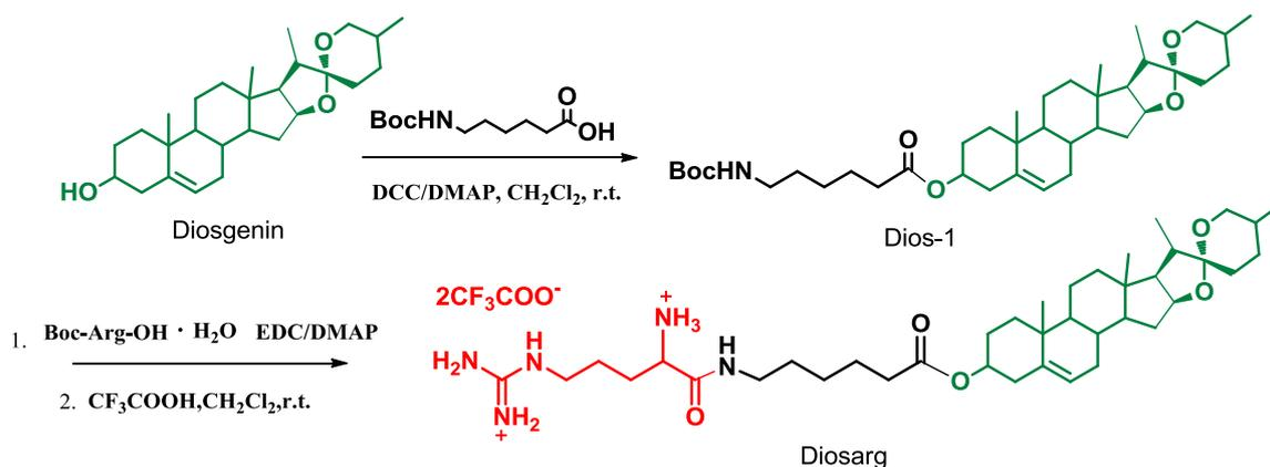
**Scheme S1.** The synthesis routes of the cationic lipid Diosarg. (DCC: N,N'-dicyclohexylcarbodiimide, EDC: 1-Ethyl-3-(3-dimethylaminopropyl)carbodiimide, DMAP: 4-Dimethylaminopyridine)
