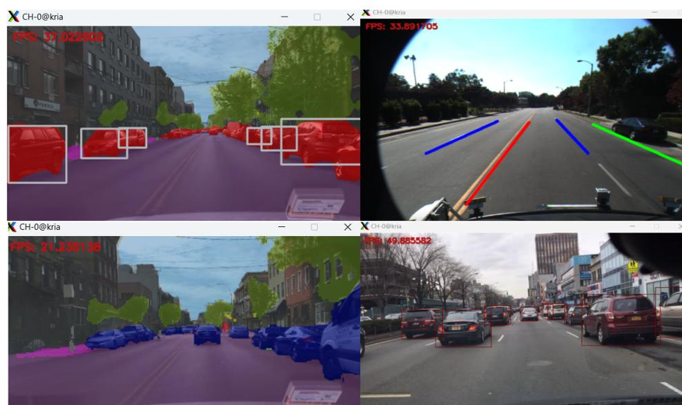
**Figure 5.** Lane detection and semantic segmentation.
