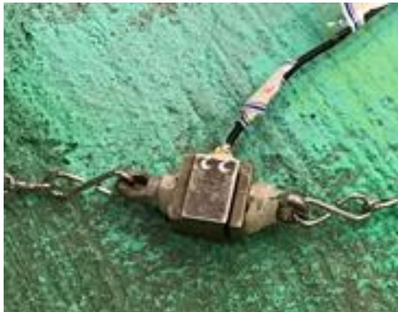
Figure 9. The load cell in the experiment.
