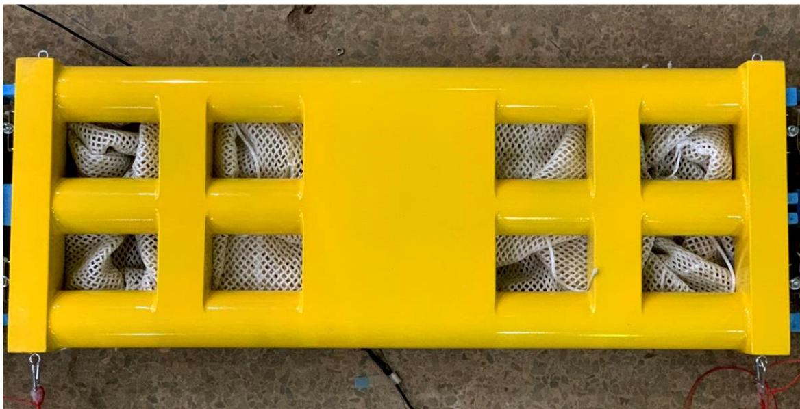
**Figure 13.** Top view of the floating breakwater model.
