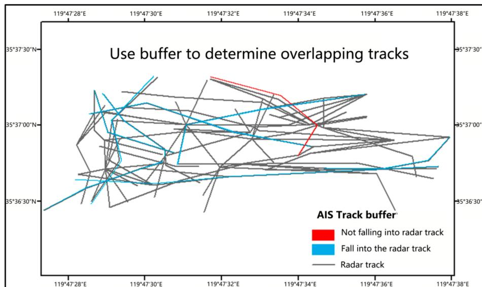
Figure 9. Using buffer to determine overlapping track results.
