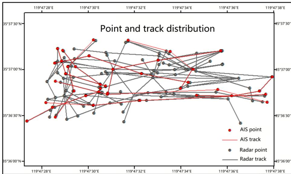
Figure 8. Points and tracks distribution of radar and AIS.
