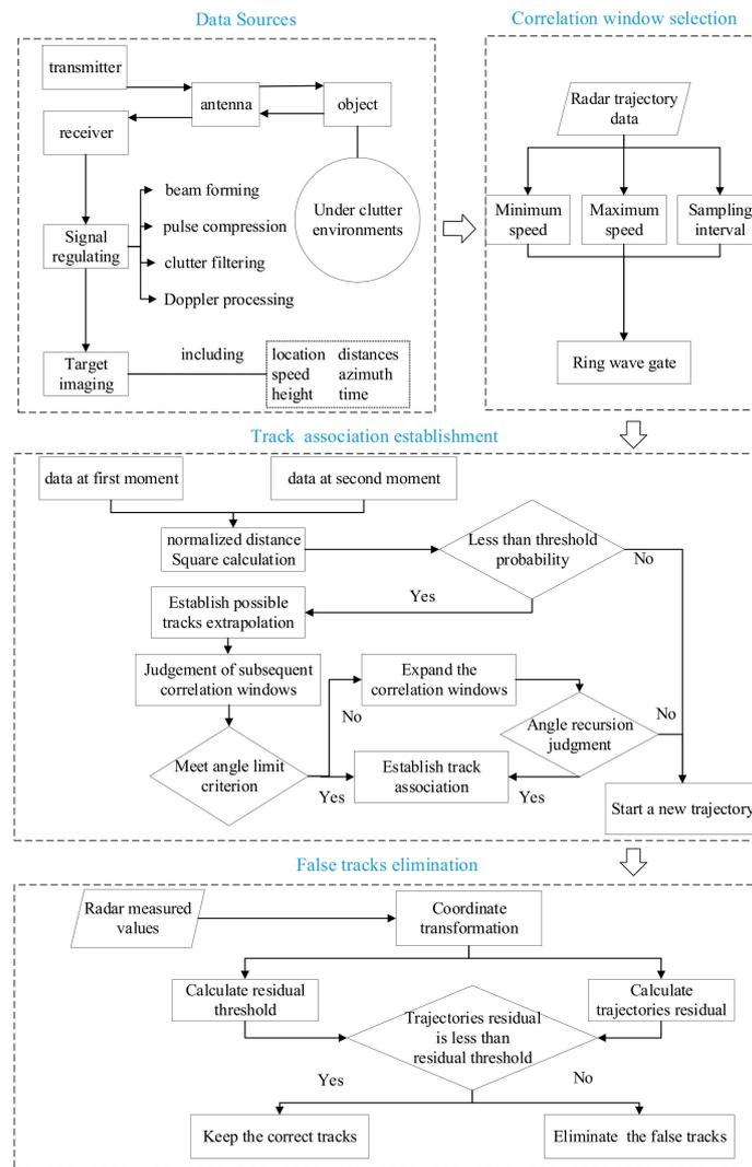
**Figure 3.** Flow chart of track initiation algorithm using the residual threshold. The data comes from the Service of State Oceanic Administration (SOA), which is processed in the process.
