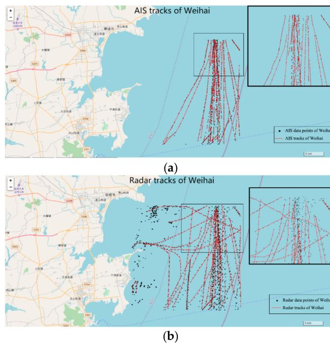
**Figure 11.** AIS tracks and radar tracks near Weihai. (a) AIS tracks of Weihai, (b) radar tracks of Weihai.
