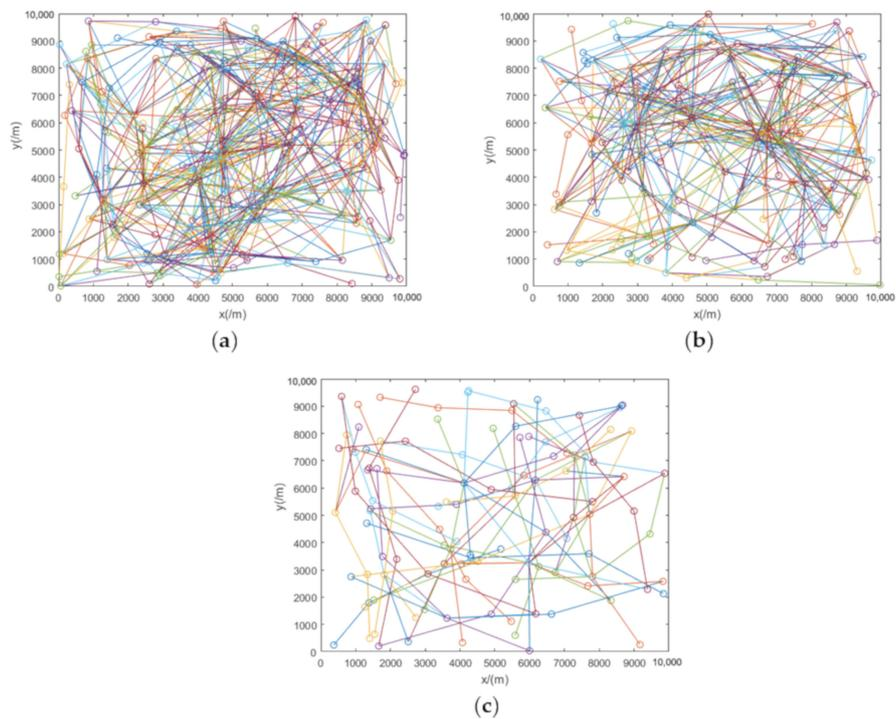
**Figure 6.** Tracks calculated by three methods: (a) is the radar track by traditional logic; (b) is the radar track by traditional Kalman filter method; (c) is the radar track by track initiation algorithm using a residual threshold.
