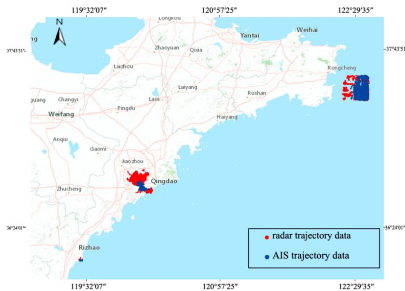
**Figure 2.** Data required for the experiment, including radar trajectory data and Automatic Identification System (AIS) trajectory data in three areas. Radar trajectory data is more than AIS trajectory data.
