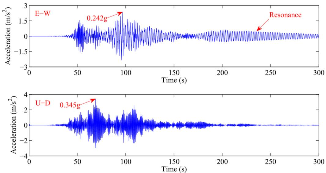
**Figure 6.** Time history of acceleration of the pipeline responding to input seismic wave. It is shown that there is a significant resonance in horizontal direction.
