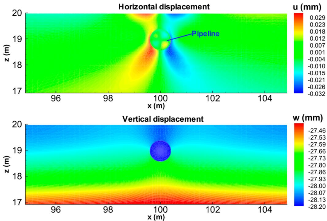
**Figure 4.** Displacement distribution of the pipeline-seabed in consolidated status. The effect of the pipeline on horizontal displacement is obvious, and the pipeline slightly subsides relative to its surrounding seabed soil.
