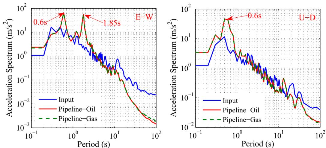
**Figure 12.** Acceleration spectrum of pipeline-gas system responding to input seismic wave. It is shown that the difference of seismic dynamics of the pipeline-oil system and the pipeline-gas system is minor.
