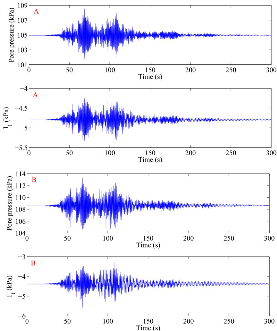
**Figure 8.** Time history of pore pressure and effective stress  $I_1$  at the two typical position A and B in the seabed foundation labelled in Figure 2. There is no residual pore pressure built in dense seabed soil.
