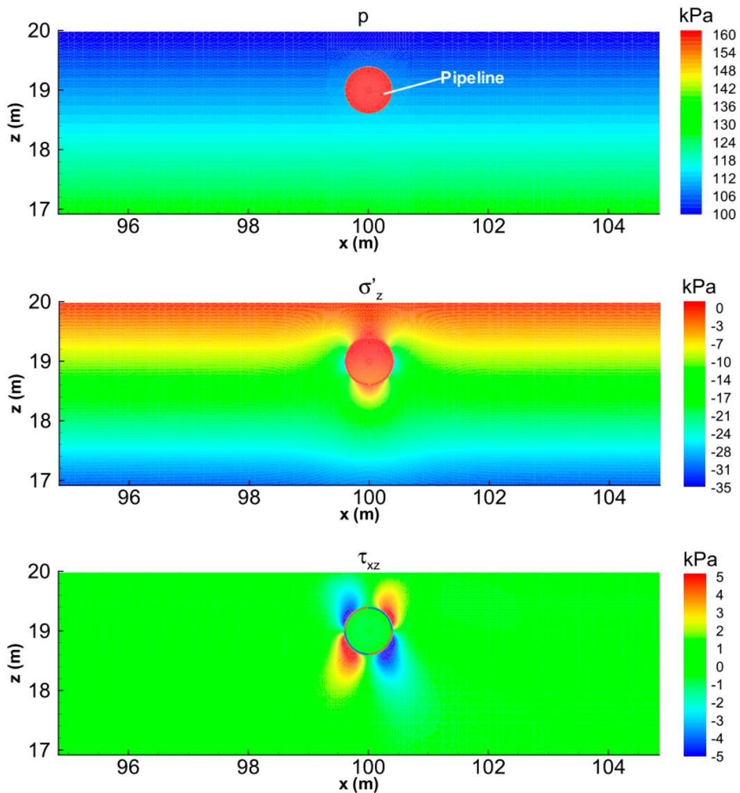
**Figure 5.** Effective stress and pore pressure distribution of the pipeline-seabed in consolidated status. The distribution of the vertical effective stress  $\sigma'_z$  indicates that an upward buoyancy is applied on the pipeline.
