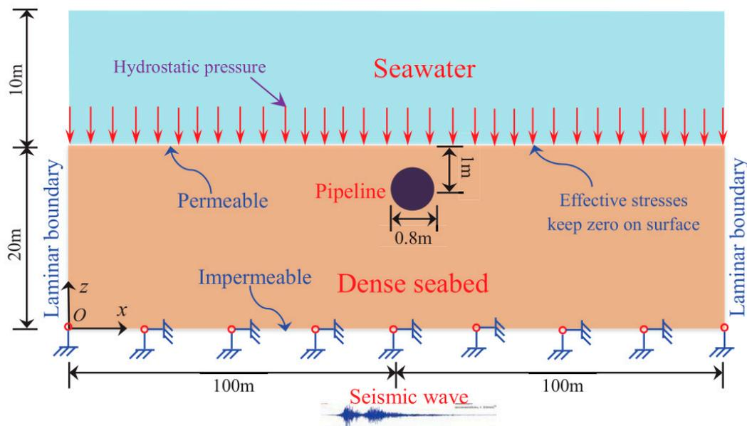
**Figure 1.** Sketch map of the pipeline-seabed system adopted in computation. A submarine pipeline is buried in the dense seabed foundation. Only the hydrostatic water pressure is applied on the surface of seabed, and the laminar boundary condition is applied on the two lateral sides.
