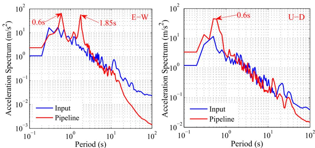
**Figure 9.** Acceleration spectrum of the pipeline responding to input seismic wave. It is observed that there are two resonance periods (0.6 s and 1.85 s) for the pipeline-crude oil-seabed foundation system.
