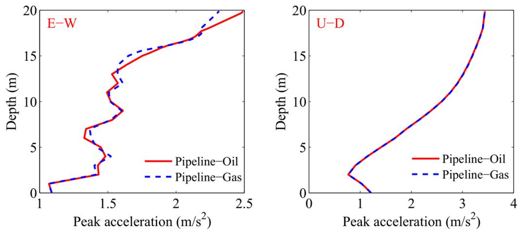
**Figure 13.** Amplification effect of the seabed soil along depth. It is confirmed that the seabed foundation has significant amplification effect to the input seismic wave in both horizontal and vertical direction.
