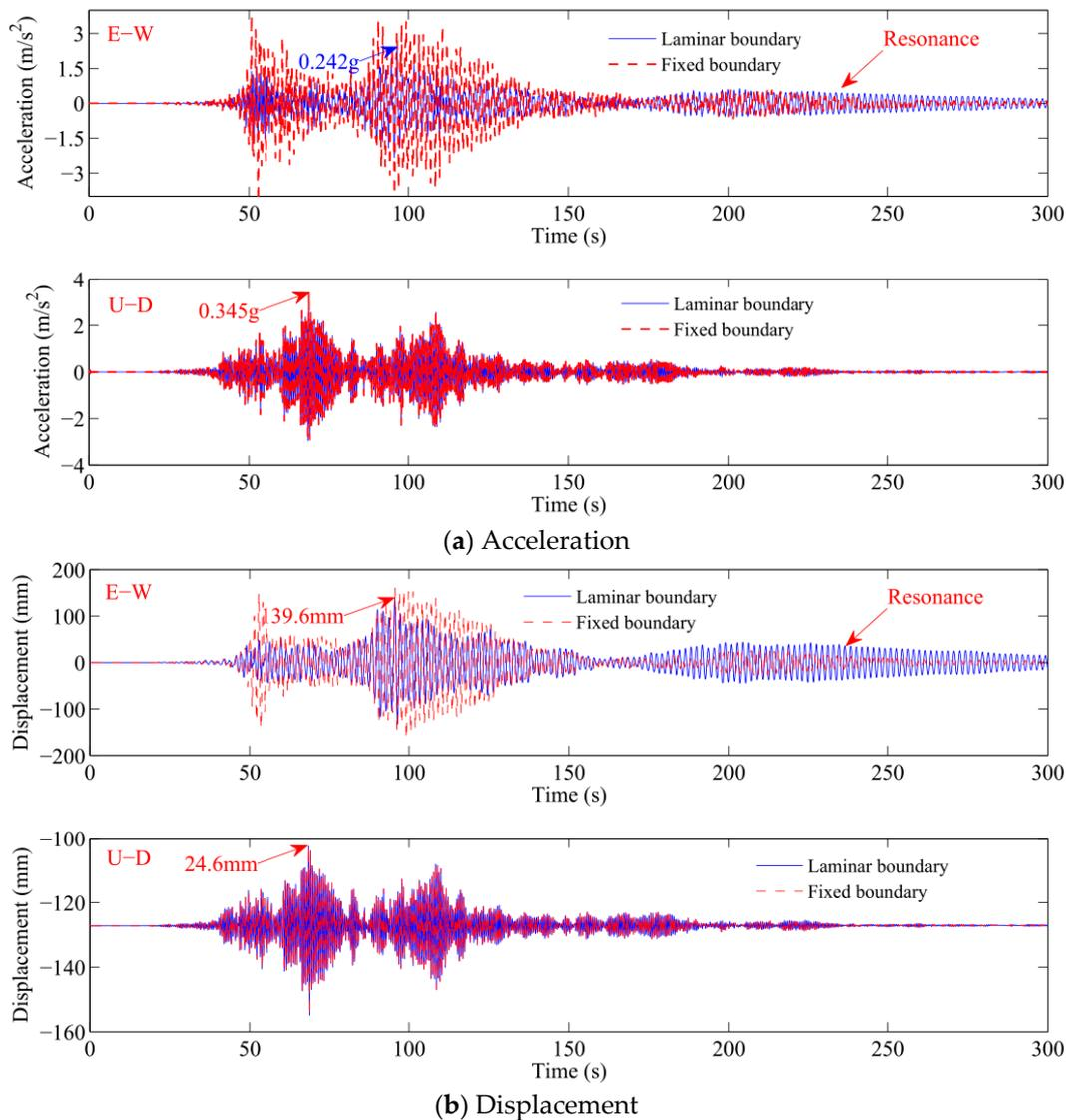
**Figure 10.** Effect of the fixed lateral side boundary on the dynamics of pipeline. It is shown that there is a significant adverse effect of the fixed lateral boundary condition on the horizontal dynamics.
