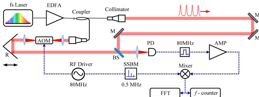
**Figure 4.** Schematic of the outdoor optical frequency transmission test system. AMP: microwave amplifiers, AOM: acousto-optic modulator, BS: beam splitter, EDFA: erbium-doped fiber amplifier, M: silver mirrors, PD: photodiode, R: retro-reflector, and SSBM: single-side band modulator.
