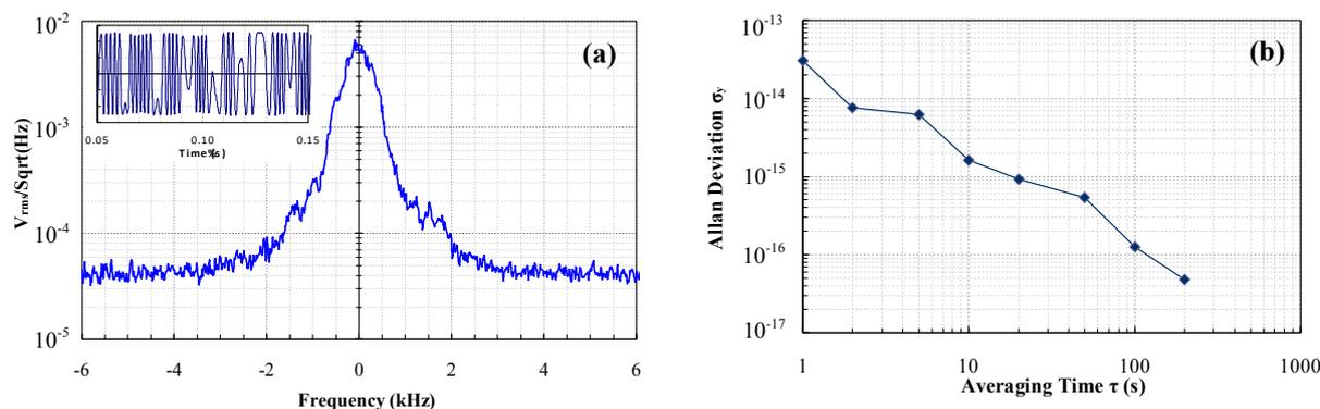
**Figure 5.** (a) A typical spectrum of the transmission-broadened optical clock signal. Inset: a time-domain trace of the beat note between the recovered clock and the original clock; (b) A typical Allan deviation measurement result.
