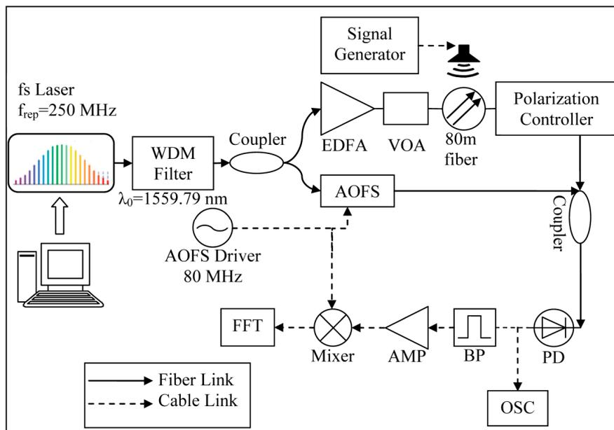
**Figure 1.** Schematic of the experimental setup for characterizing the excess phase noise spectra of optical frequency transfer in a fiber link under external acoustic perturbations. AMP, microwave amplifier; BP, band pass filter; OSC, oscilloscope; WDM, wavelength division multiplexer.
