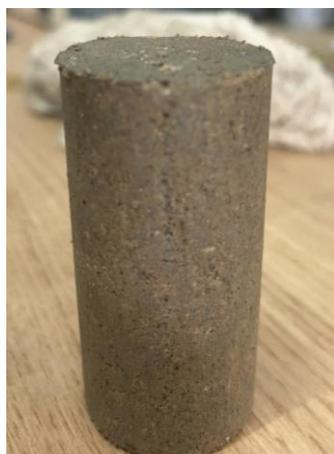
**Figure 5.** Specimen of granite residual soil amended with fly ash.
