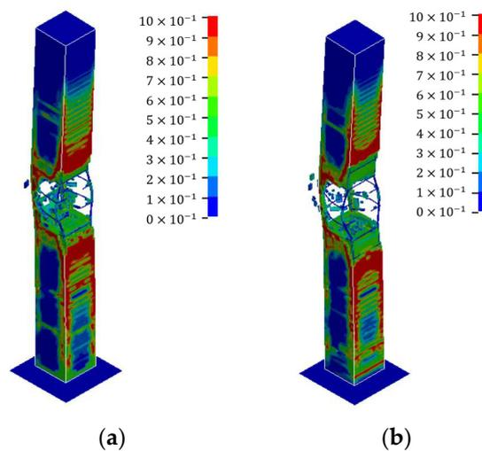
Figure 5. Damage diagram of the reinforced concrete column. (a) is the damage diagram for the Z4-1 condition; (b) is the damage diagram for the Z5-1 condition.
