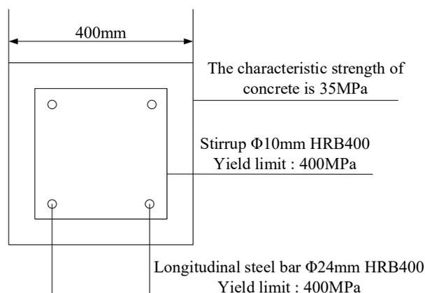
**Figure 3.** Reinforcement diagram of the reinforced concrete column.
