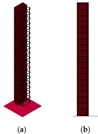
**Figure 4.** Mesh model of the reinforced concrete column. (a) is a 45 ° view of the cylinder; (b) is the side view of the cylinder.
