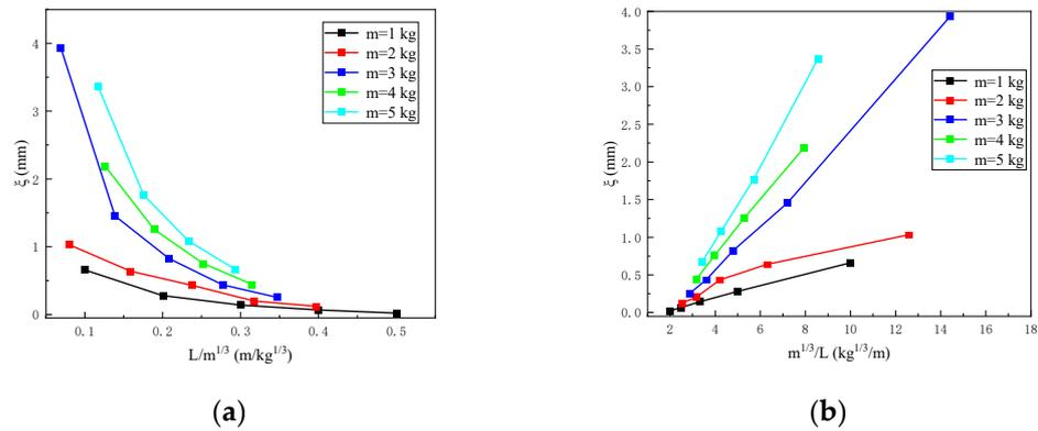
**Figure 6.** The relationship between the disturbance and the explosion distance and the explosion equivalent in the column under different explosion equivalents. (a) is the change curve of  $\xi$  and  $L/m^{1/3}$ ; (b) is the change curve of  $\xi$  and  $m^{1/3}/L$ .
