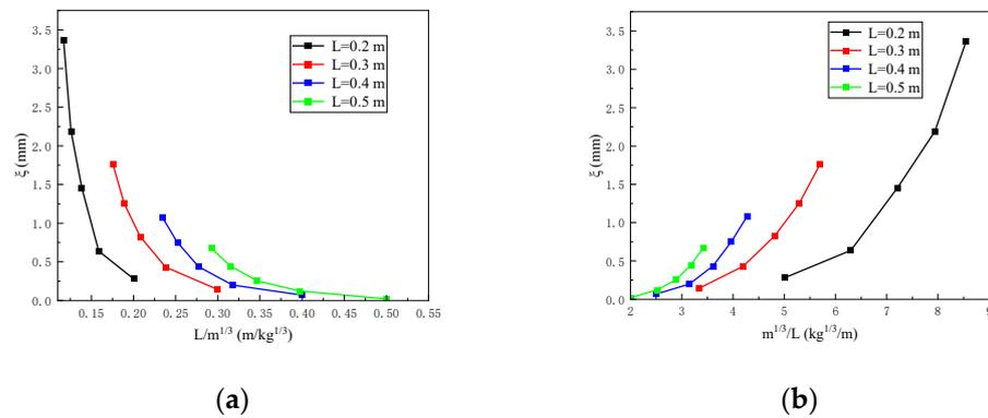
**Figure 7.** The relationship between the disturbance in the column and the explosion distance and the explosion equivalent under different explosion distances. (a) is the change curve of  $\xi$  and  $L/m^{1/3}$ ; (b) is the change curve of  $\xi$  and  $m^{1/3}/L$ .
