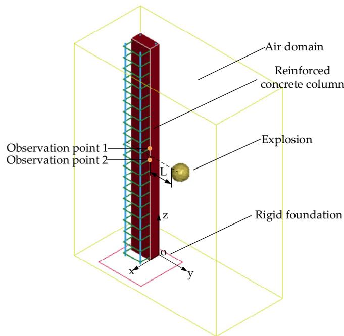
**Figure 1.** Damage diagram of a reinforced concrete column.
