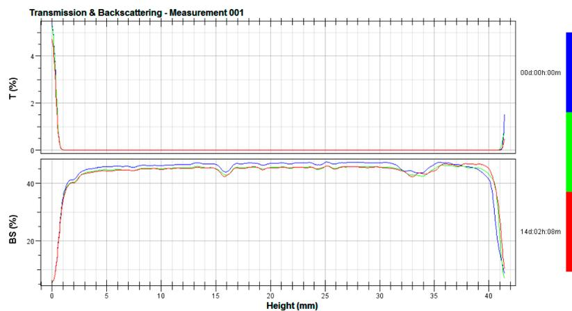
**Figure A6.** Dependence of transmittance (T) and back scattering (BS) on sample height for a prototype HC\_6; dark blue line—evaluation of the preparation immediately after application into tubes (time “0”), green line—stability after 7 days, red line—stability after 14 days.
