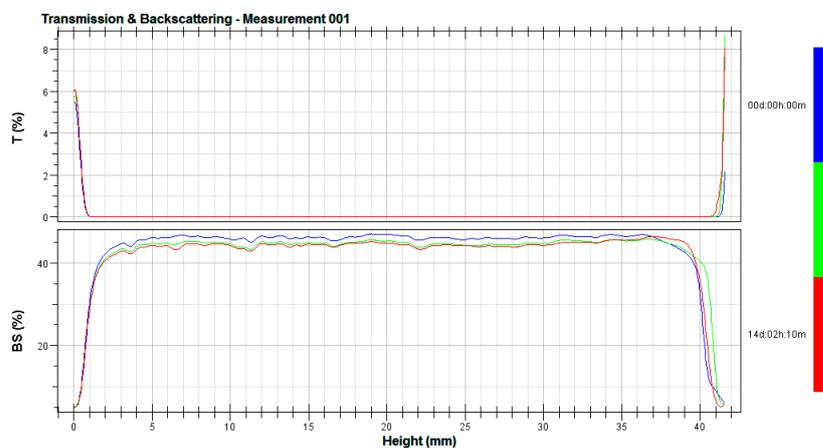
**Figure A5.** Dependence of transmittance (T) and back scattering (BS) on sample height for a prototype HC\_5; dark blue line—evaluation of the preparation immediately after application into tubes (time “0”), green line—stability after 7 days, red line—stability after 14 days.
