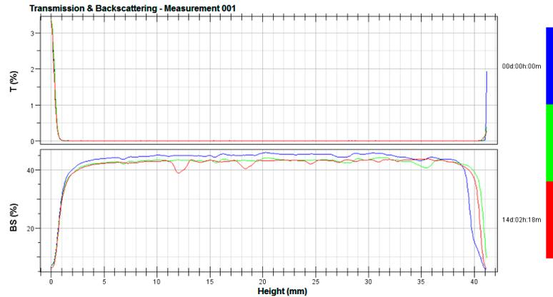
**Figure A1.** Dependence of transmittance (T) and back scattering (BS) on sample height for a prototype HC\_1; dark blue line—evaluation of the preparation immediately after application into tubes (time “0”), green line—stability after 7 days, red line—stability after 14 days.
