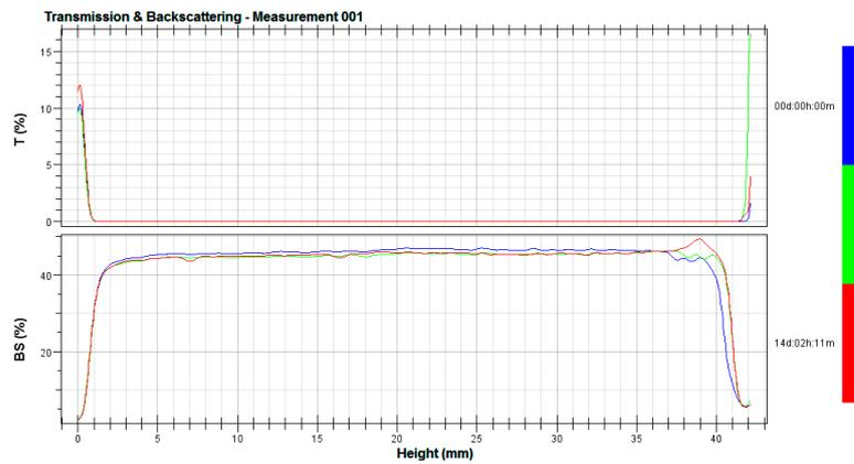
**Figure A2.** Dependence of transmittance (T) and back scattering (BS) on sample height for a prototype HC\_2; dark blue line—evaluation of the preparation immediately after application into tubes (time “0”), green line—stability after 7 days, red line—stability after 14 days.
