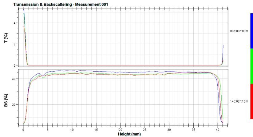
**Figure A4.** Dependence of transmittance (T) and back scattering (BS) on sample height for a prototype HC\_4; dark blue line—evaluation of the preparation immediately after application into tubes (time “0”), green line—stability after 7 days, red line—stability after 14 days.
