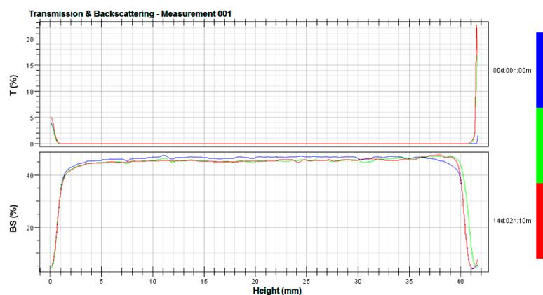
**Figure A3.** Dependence of transmittance (T) and back scattering (BS) on sample height for a prototype HC\_3; dark blue line—evaluation of the preparation immediately after application into tubes (time “0”), green line—stability after 7 days, red line—stability after 14 days.
