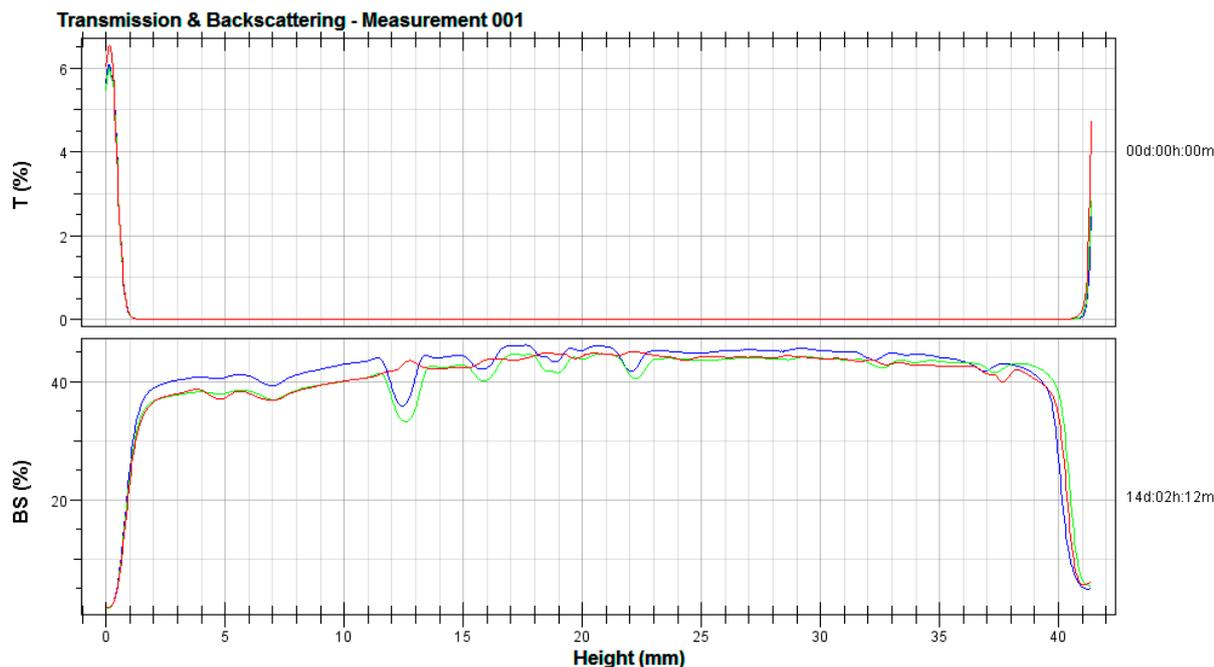
**Figure 2.** Dependence of transmittance (T) and back scattering (BS) on sample height for a prototype HC\_0; dark blue line—evaluation of the preparation immediately after application into tubes (time “0”), green line—stability after 7 days, red line—stability after 14 days.
