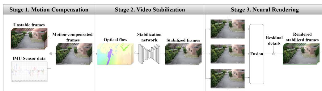
**Figure 4.** The overall pipeline of the proposed cross-interaction-based hybrid full-frame video stabilization framework. (**Stage 1**) We first perform motion compensation using IMU sensor data. (**Stage 2**) Then, the motion compensated frames are estimated using the optical flow and these are input into a stabilization network to create stabilized frames. (**Stage 3**) Finally, multiple frames are fused and residual details are combined to generate the final rendered stabilized frames.
