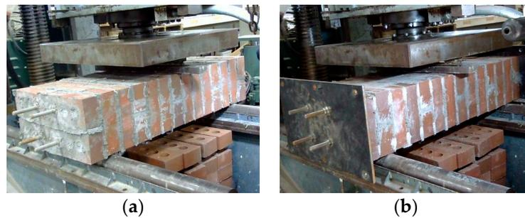
Figure 8. 3-point bending test in this study: (a) Example of IRBM; (b) Example of IRBM—F.
