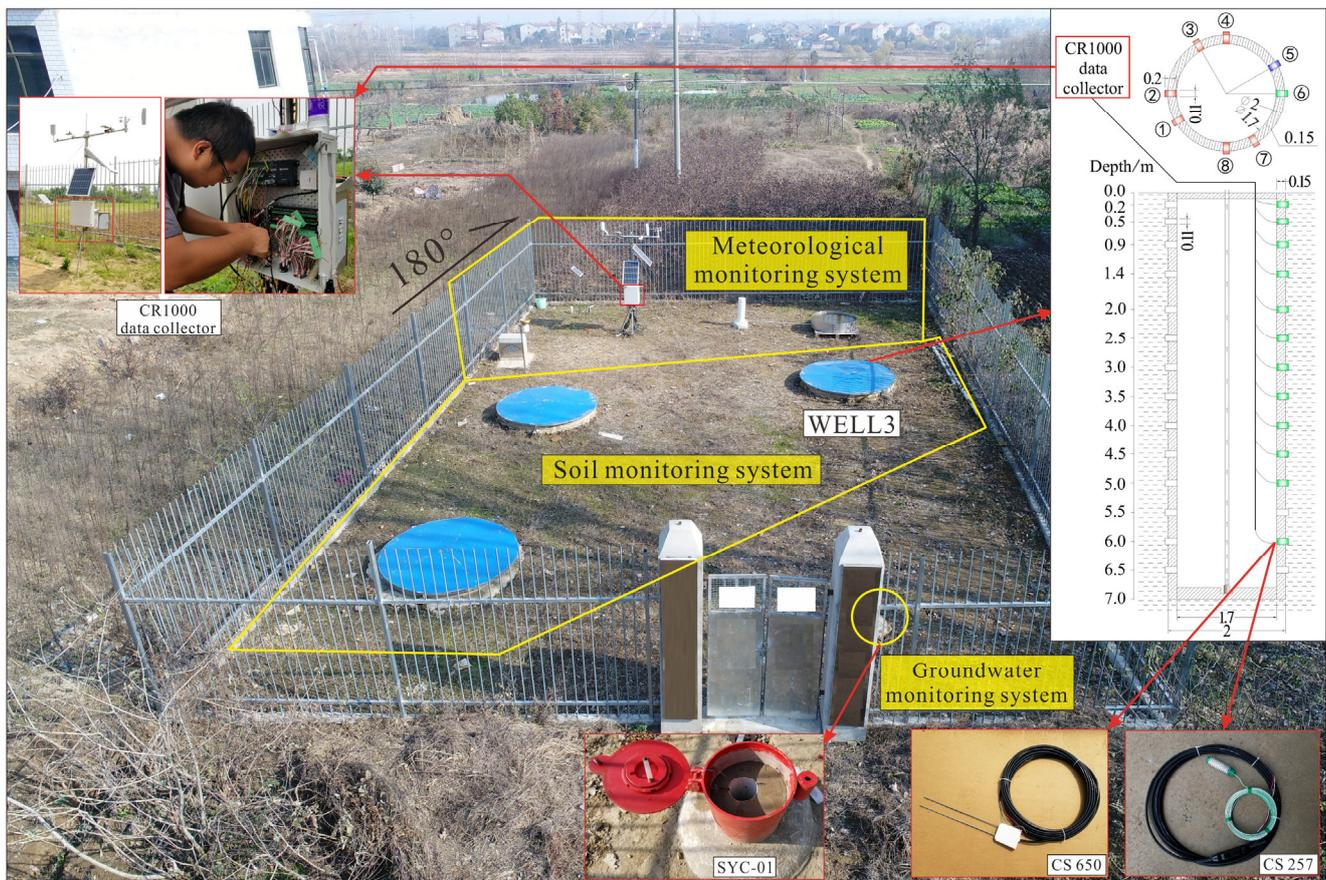
**Figure 1.** Monitoring and data collection systems of the field test site. The number “①–⑧” in the north-eastern part of this figure are the numbers of horizontal holes for instrument installation. The CS257 and CS650 probes were installed inside holes “⑤–⑥” at the east direction of WELL3.
