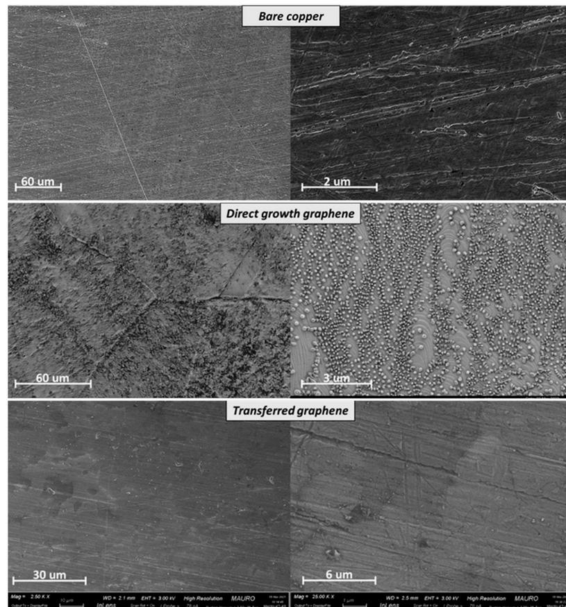
**Figure 2.** SEM imaging of transferred and directly grown graphene with magnification 500×, 2.5 kX and 25 kX.
