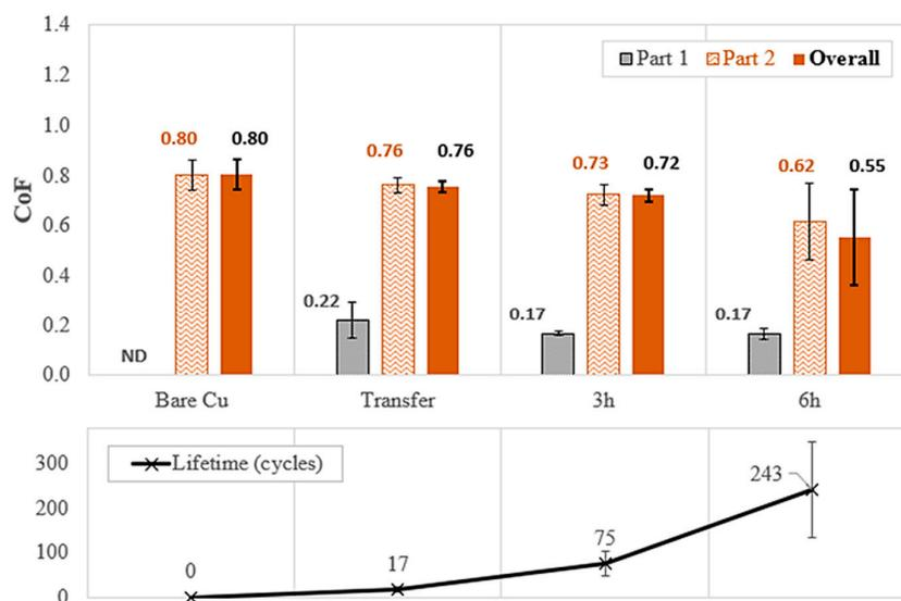
**Figure 9.** Average CoF values measured in Part 1 and Part 2. The error bars were determined as three times the standard deviation of the average CoF of the three tests carried out with each sample (Lower part). Average lifetime of the coatings determined by the cycles accumulated at the time the transition from Part 1 to Part 2 started.
