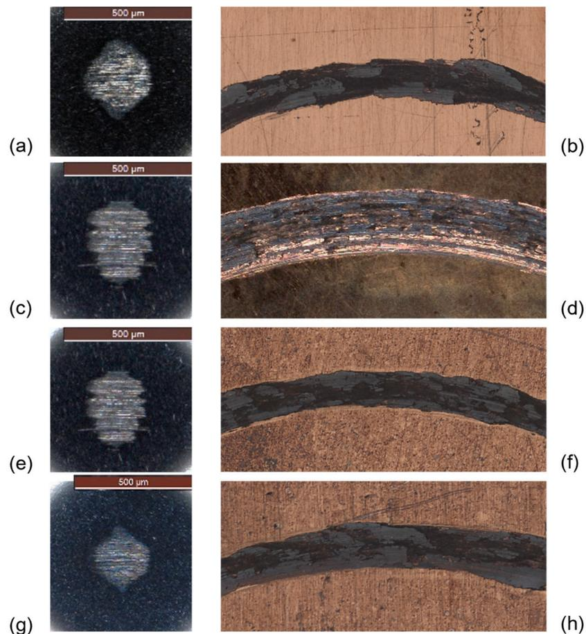
**Figure 14.** (a) Wear scars on the steel balls (left) and wear tracks on the copper samples (right). (a,b) Bare Cu, (c,d) transferred graphene, (e,f) 3 h-sonicated graphene, (g,h) 6 h-sonicated graphene.
