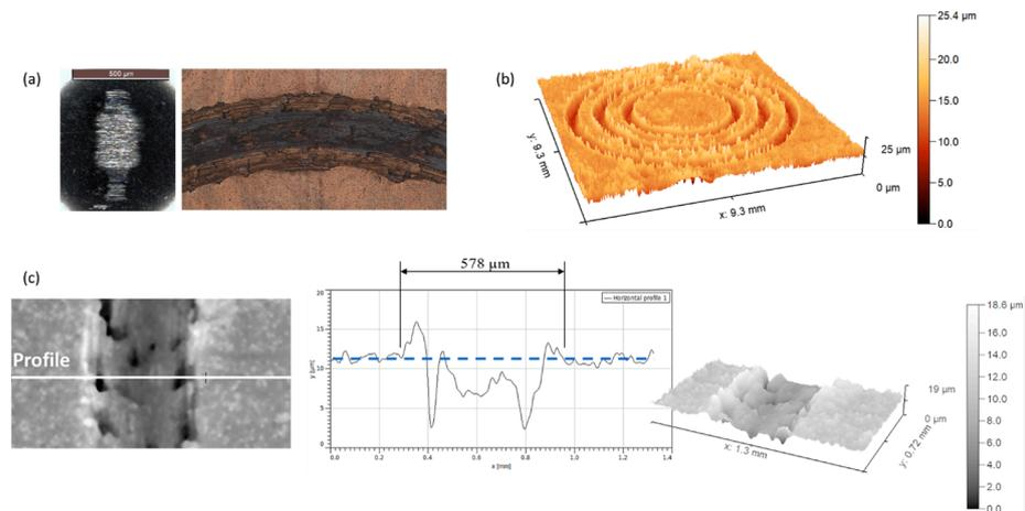
**Figure 17.** Morphological analysis of the wear track after the tribological test with the sample treated by direct growth CVD. (a) chunks of material ripped off the samples, (b) 3D measurement, (c) wear track measurement.
