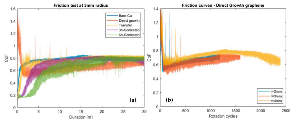
**Figure 15.** (a) Friction curves were measured with the sample treated by direct growth CVD and compared to the other samples at the median radius of 3 mm. (b) Set of friction curves measured with the direct growth sample.
