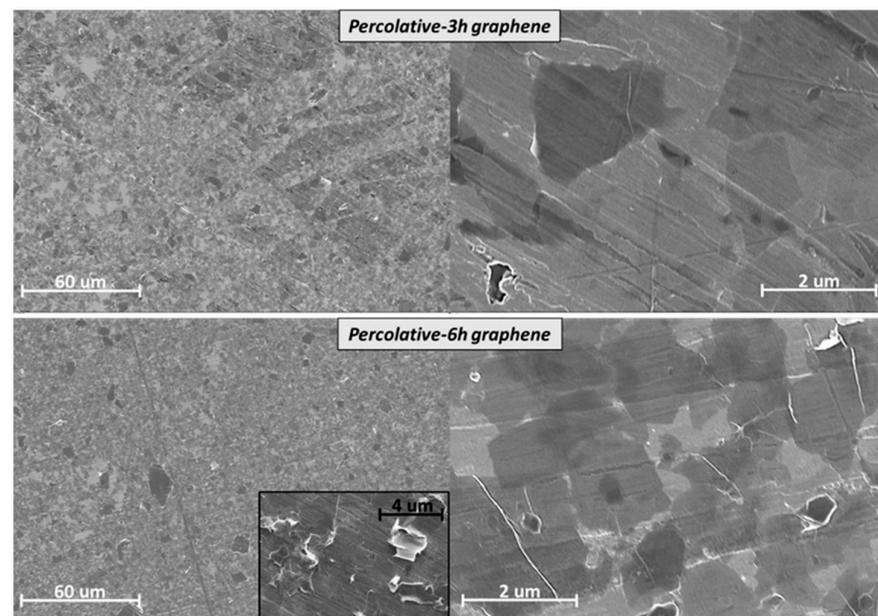
**Figure 3.** SEM imaging of the percolative graphene nano-coatings with magnification  $500\times$  and  $15\text{ kX}$ . Inset shows defective recombination of GNPs resulting from the production process of the graphene sheet.
