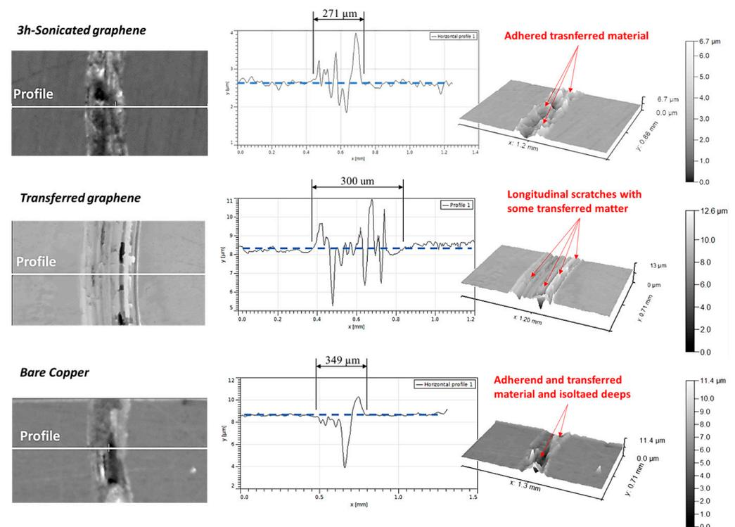
**Figure 13.** Analysis of the wear tracks morphology. The wear tracks of the tests performed at 3 mm radius were considered for this comparative analysis.
