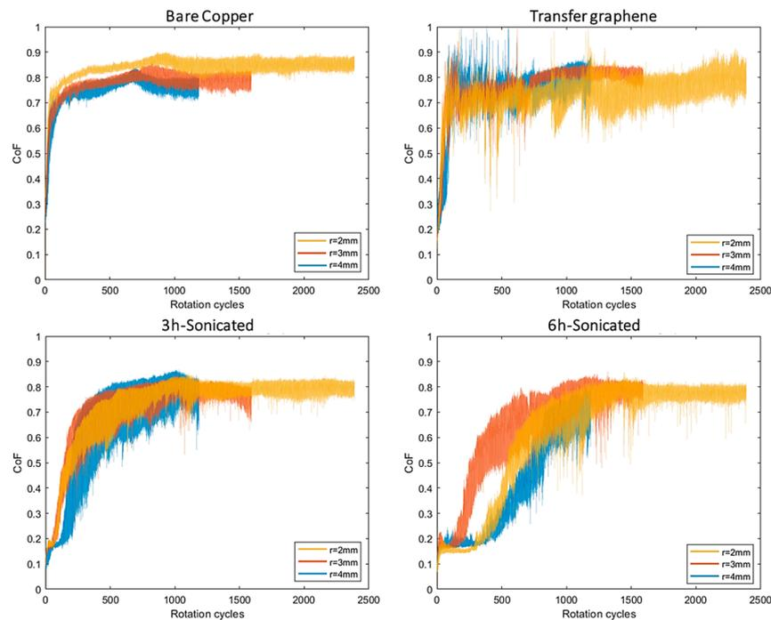
**Figure 8.** Friction curves from pin-on-disc tests on the graphene-coated samples. Friction curves plotted against the number of rotation cycles allows appreciating the high repeatability of the results despite the different wear track radii.
