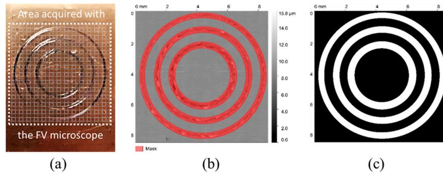
**Figure 5.** (a) Region of the samples scanned with the 3D microscope, (b) masks applied to the topographic data, (c) binary trace of the masked region.
