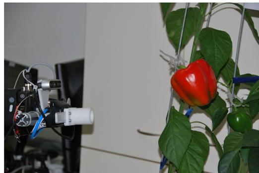
**Figure 3.** Camera mounted on robotic arm acquiring images of red sweet pepper mounted on a pepper plant.
